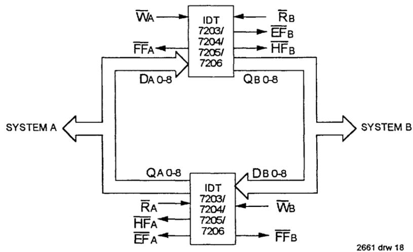
Figure 16. Bidirectional FIFO Operation
