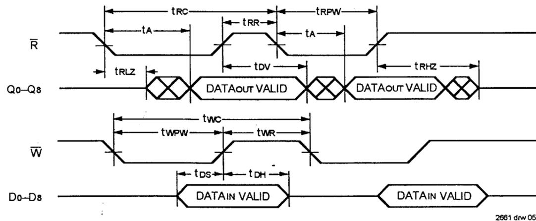
Figure 3. Asynchronous Write and Read Operation
