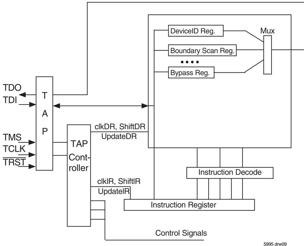
Figure 6. Boundary Scan Architecture
