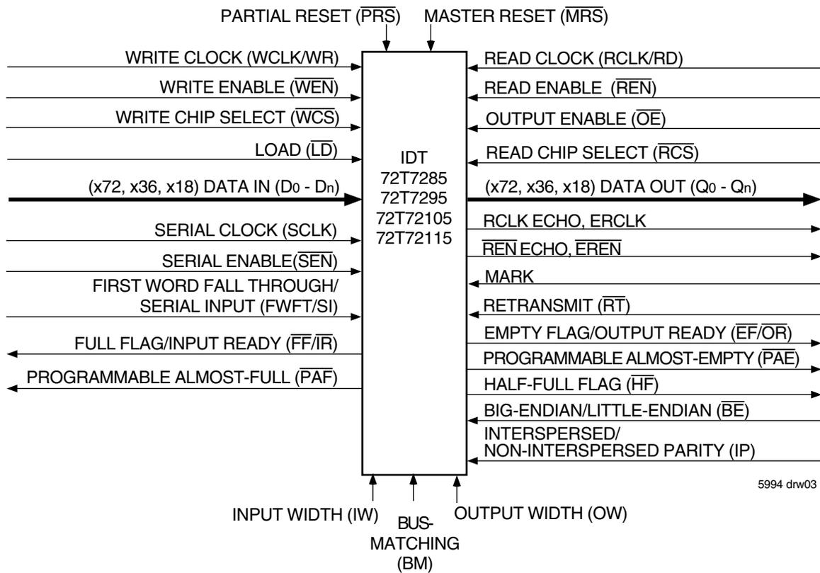
Figure 1. Single Device Configuration Signal Flow Diagram
