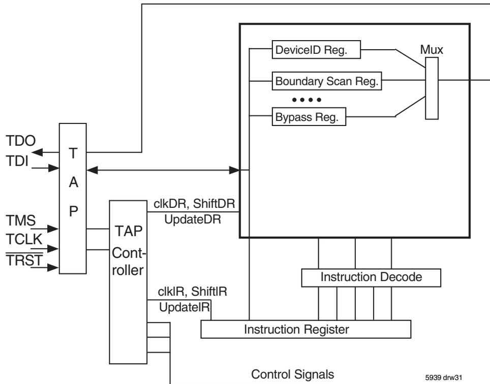
Figure 29. Boundary Scan Architecture
