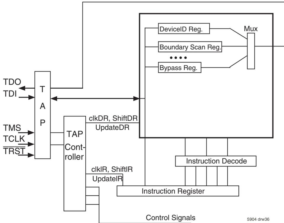
Figure 33. Boundary Scan Architecture
