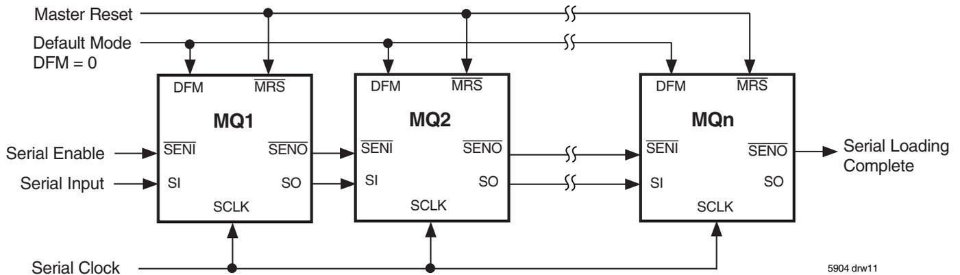
Figure 6. Serial Port Connection for Serial Programming
