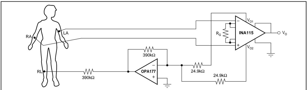
FIGURE 7. ECG Amplifier with Right Leg Drive.
