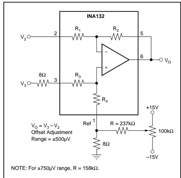
FIGURE 2. Offset Adjustment.
