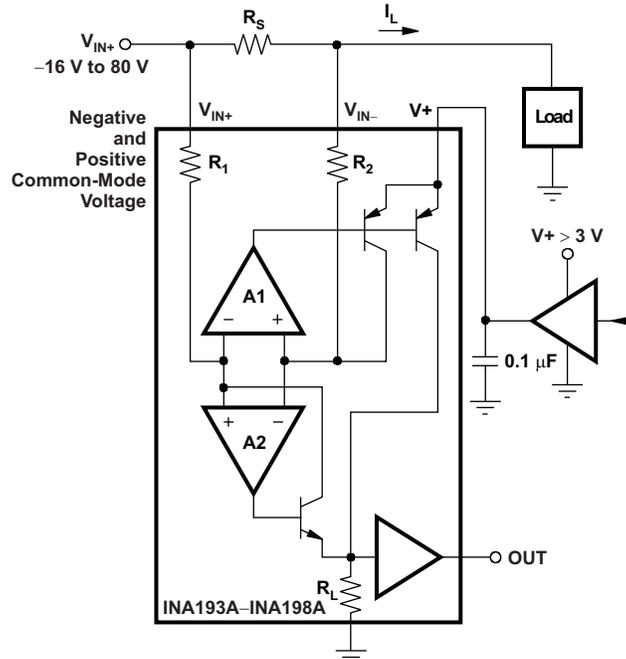
**Figure 4. INA193A–INA198A Example Shutdown Circuit**
