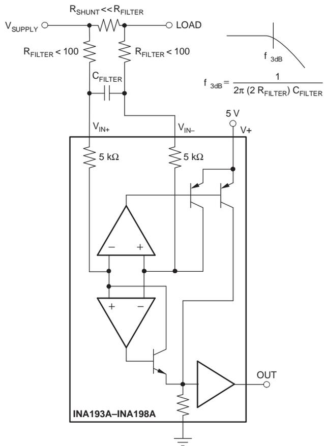
Figure 5. Input Filter (Gain Error = 1.5% to –2.2%)
