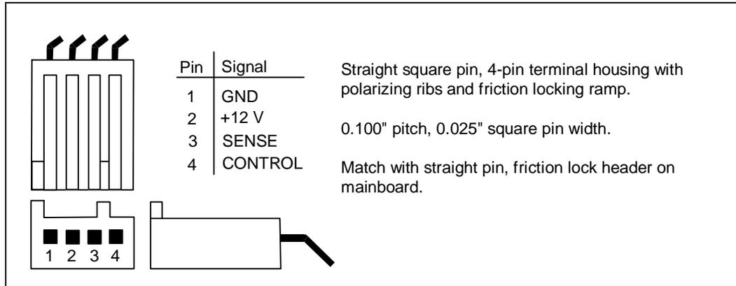
Table 30. Fan Heatsink Power and Signal Specifications
