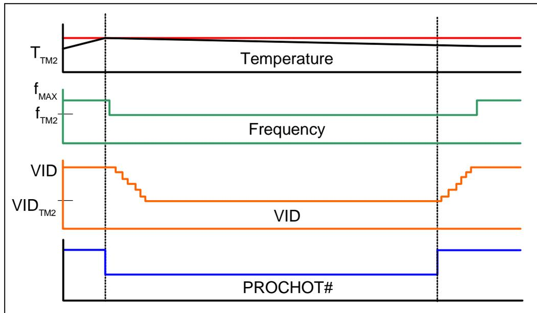
The PROCHOT# signal is asserted when a high temperature situation is detected, regardless of whether Thermal Monitor or Thermal Monitor 2 is enabled.
