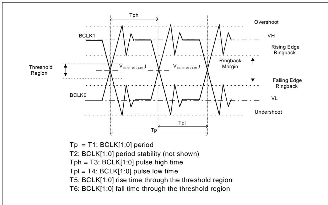
Figure 4. Measurement Points for Differential Clock Waveforms
