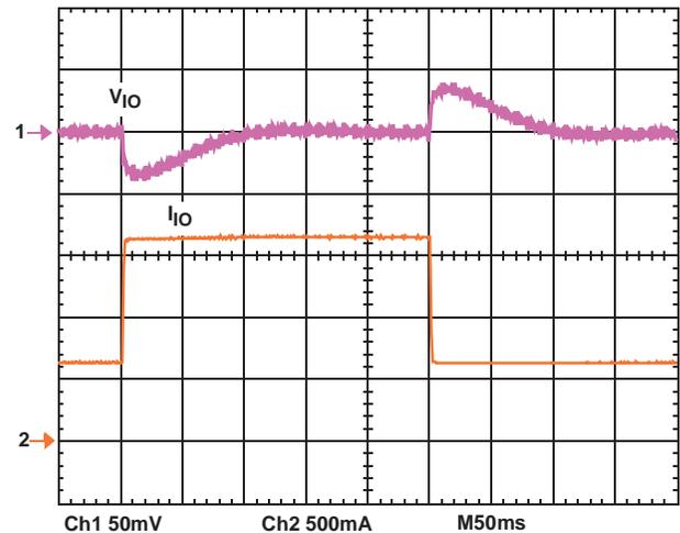
FIGURE 9. I/O CONVERTER LOAD TRANSIENT IN PWM MODE
