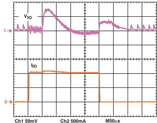
FIGURE 10. I/O CONVERTER LOAD TRANSIENT WITH MODE CHANGE
