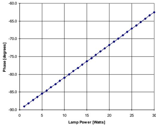
Figure 4, Lamp power vs. phase of output stage.
