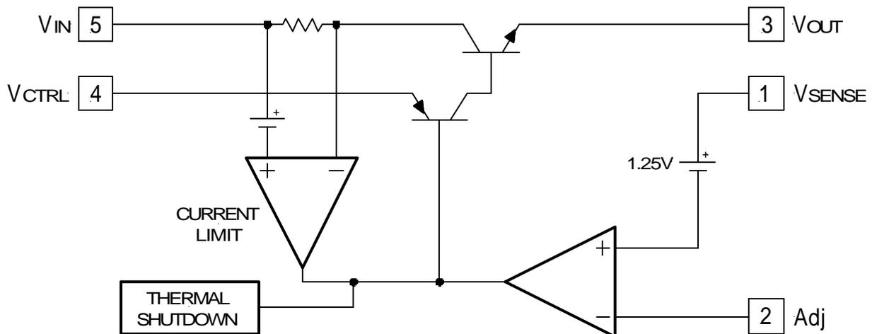
Figure 2 - Simplified block diagram of the IRU1160.
