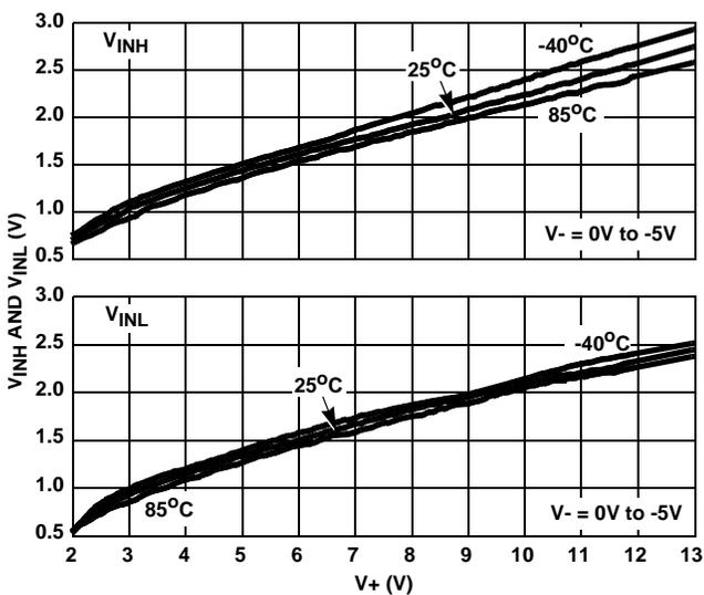
FIGURE 17. DIGITAL SWITCHING POINT vs POSITIVE SUPPLY VOLTAGE
