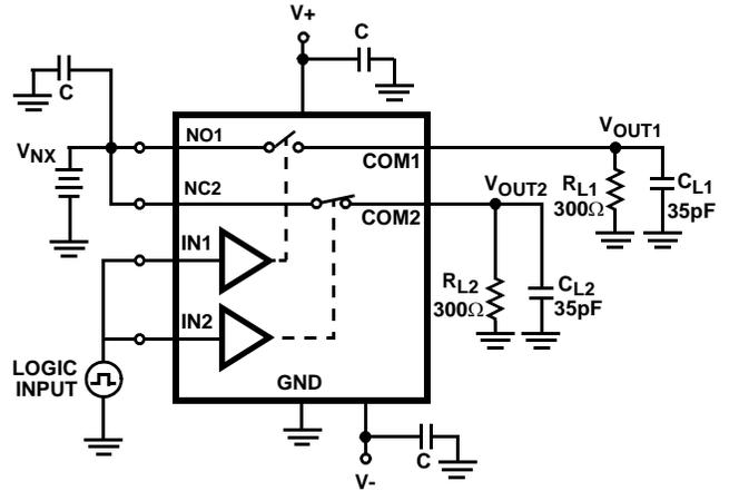
$C_L$  includes fixture and stray capacitance.
