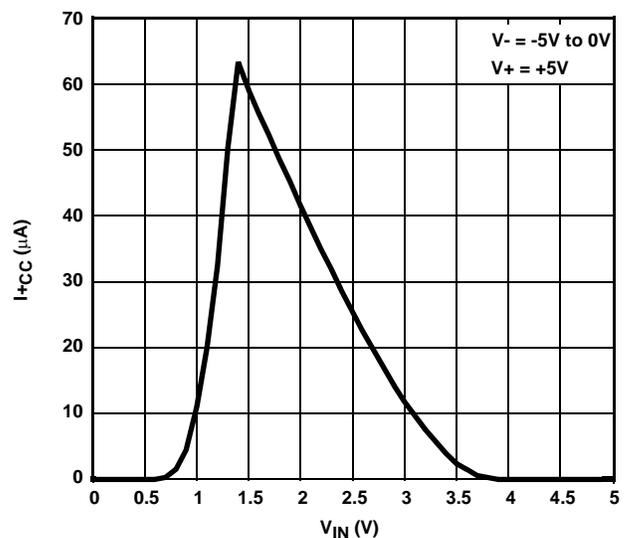
FIGURE 18. POSITIVE SUPPLY CURRENT vs DIGITAL INPUT VOLTAGE
