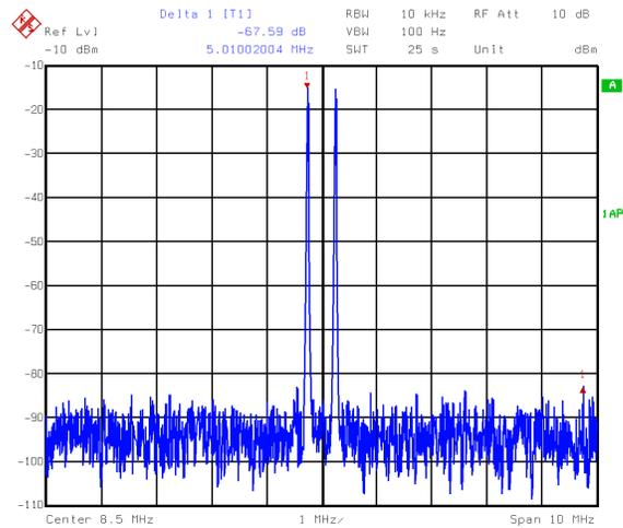
**FIGURE 4. TWO TONES (CF=6) AT 8.5MHz, 50MSPS CLOCK,**
