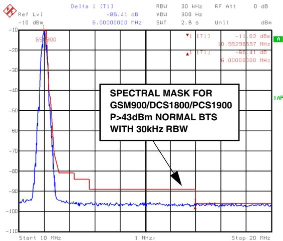
**FIGURE 3. GSM AT 11MHz, 78MSPS CLOCK**
