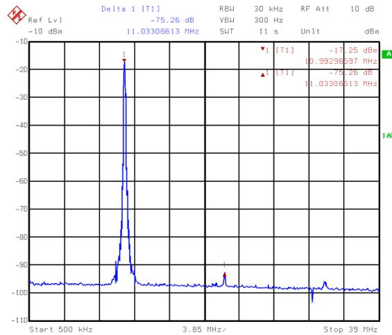
**FIGURE 2. EDGE AT 11MHz, 78MSPS CLOCK**
