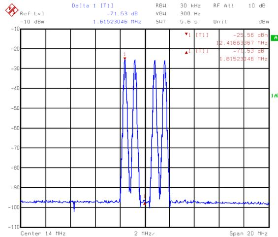
**FIGURE 6. FOUR GSM CARRIERS AT 12.4–15.6MHz,**
