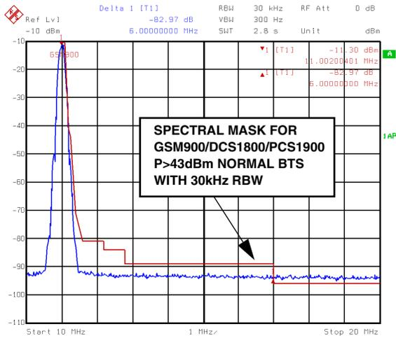
**FIGURE 1. EDGE AT 11MHz, 78MSPS CLOCK**
