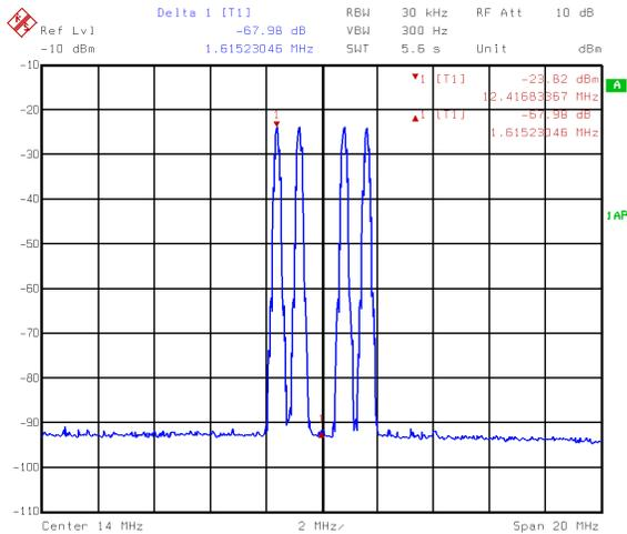
**FIGURE 5. FOUR EDGE CARRIERS AT 12.4–15.6MHz,**
