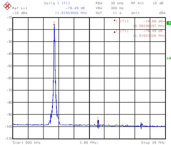
**FIGURE 4. GSM AT 11MHz, 78MSPS CLOCK**
