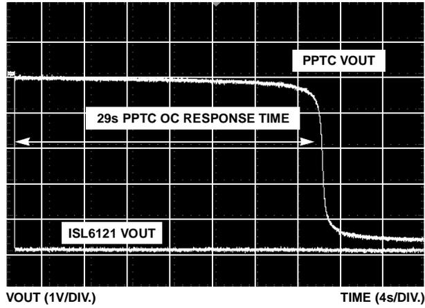
FIGURE 16. ISL6121 vs PPTC WITH EXTENDED 1.6Ω LOAD
