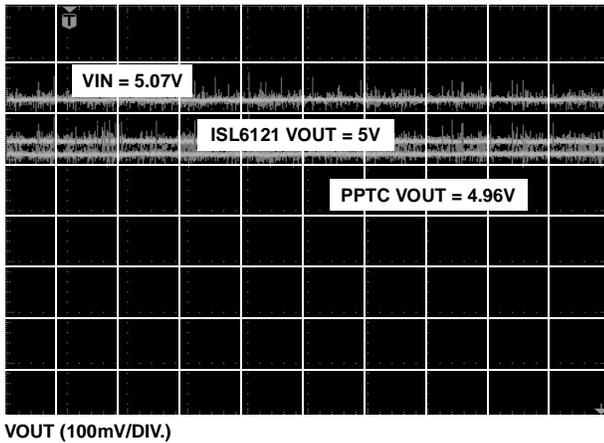
FIGURE 14. ISL6121 vs PPTC INTO 3.3Ω LOAD
