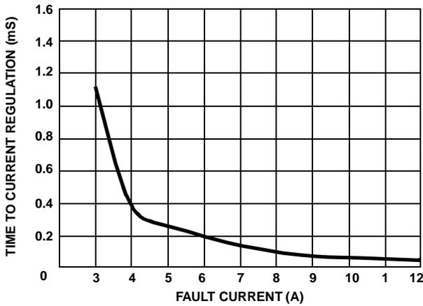
FIGURE 8. CR SETTling TIME vs FAULT CURRENT
