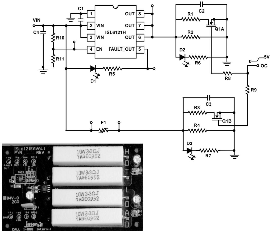
FIGURE 17. ISL6121EVAL1 SCHEMATIC AND PHOTOGRAPH
