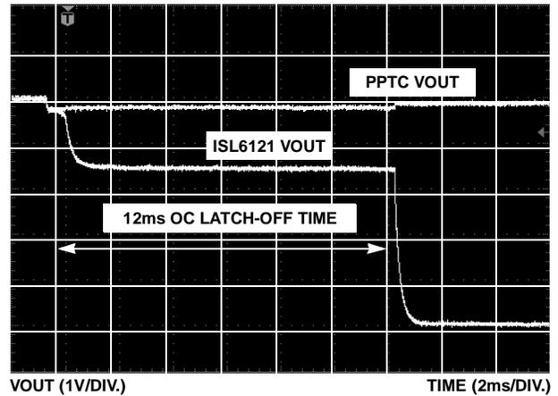
FIGURE 15. ISL6121 vs PPTC INTO 1.6Ω LOAD
