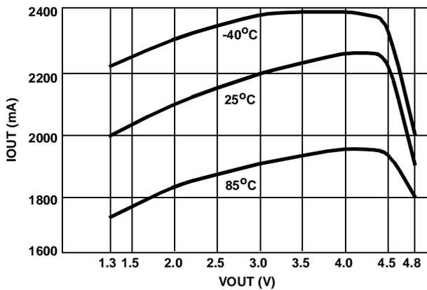
FIGURE 6. CURRENT REGULATION vs VOUT (VIN = 5.0V)
