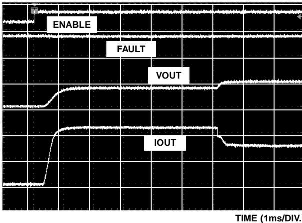
FIGURE 12. ISL6121 TURN-ON INTO A 6ms MOMENTARY OC
