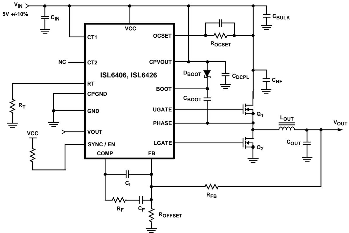
Typical Application Schematic for 3.3V Input
