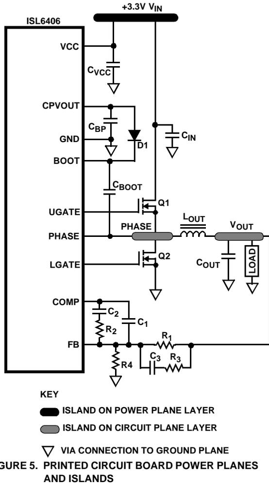
The critical small signal components include any bypass capacitors, feedback components, and compensation components. Position the bypass capacitor,  $C_{BP}$ , close to the VCC pin with a via directly to the ground plane. Place the PWM converter compensation components close to the FB and COMP pins. The feedback resistors for both regulators should also be located as close as possible to the relevant FB pin with vias tied straight to the ground plane as required.
