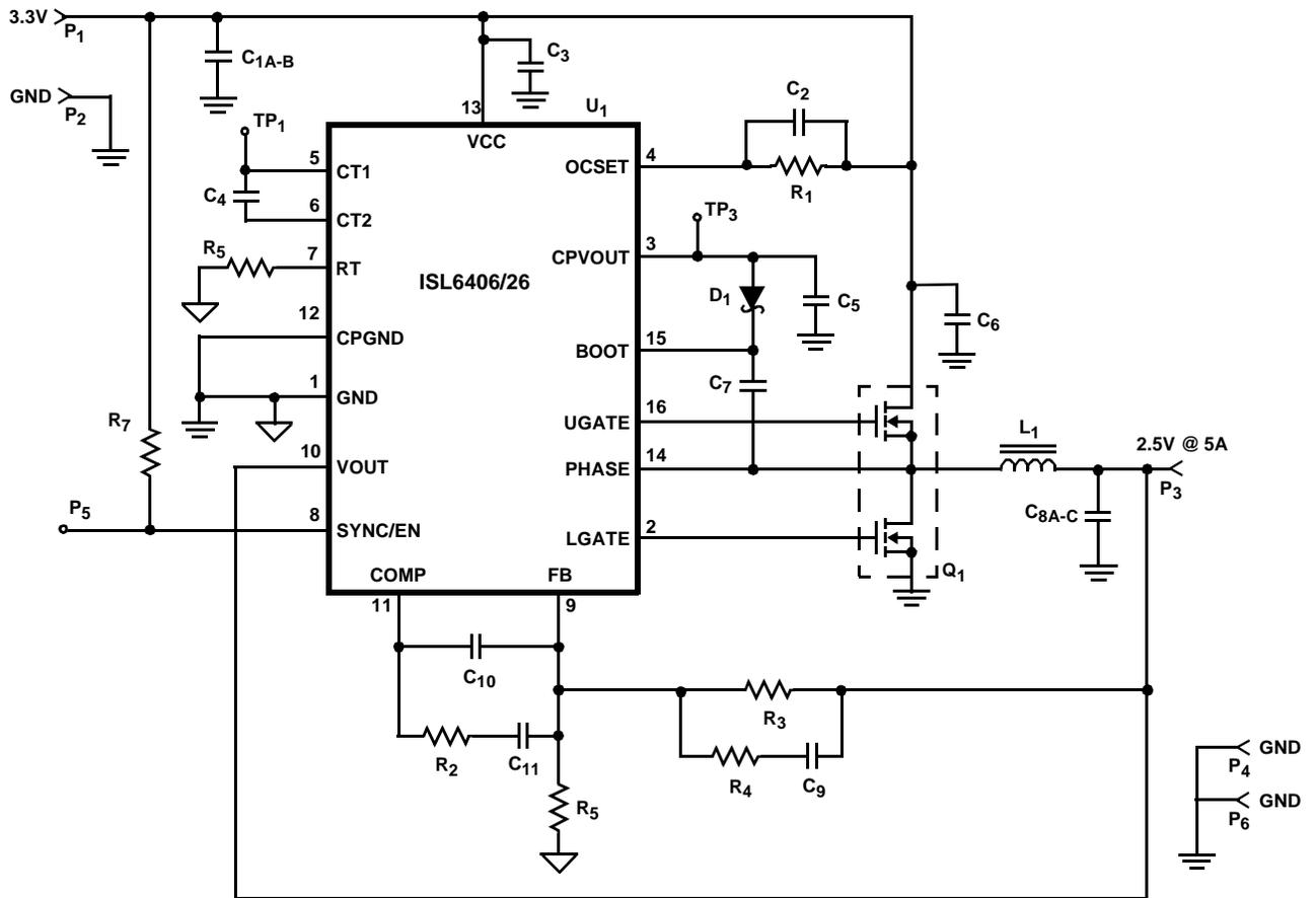
NOTE: Remove R3, R4, C9, and R5 from the board for ISL6426 evaluation.
