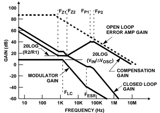
FIGURE 8. ASYMPTOTIC BODE PLOT OF CONVERTER GAIN
