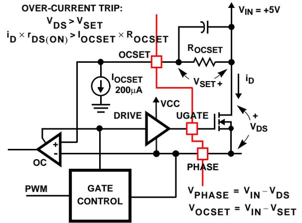
FIGURE 9. OVER-CURRENT DETECTION
