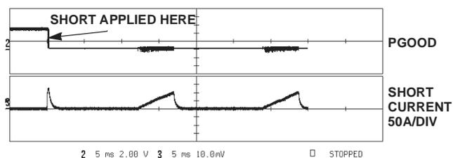
HICUP MODE. SUPPLY POWERED BY ATX SUPPLY
