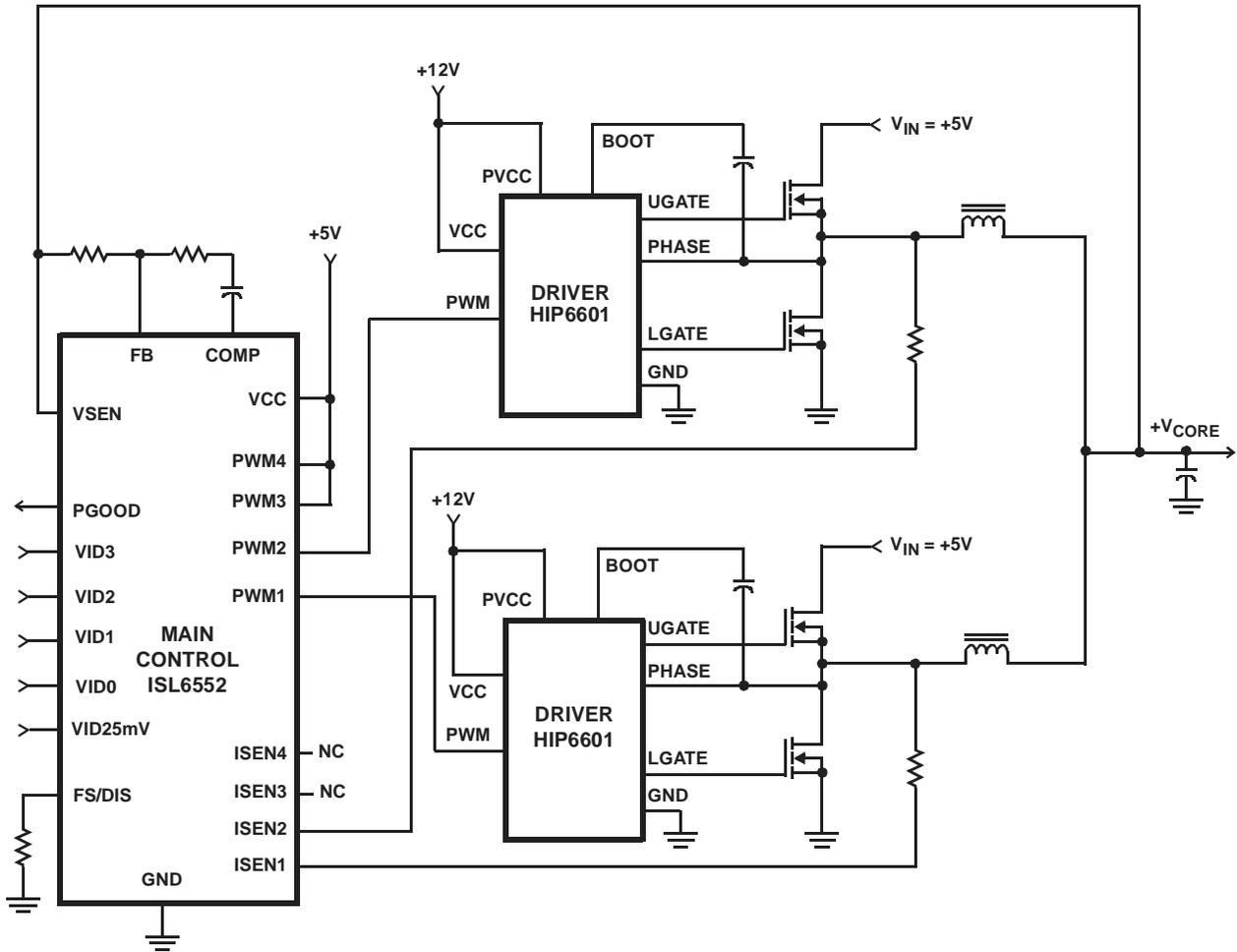
Typical Application - 4 Phase Converter Using HIP6602 Gate Drivers
