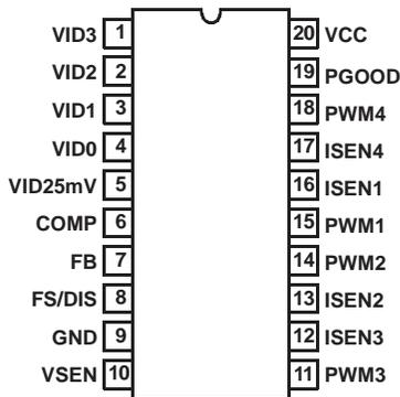
**VID3 (Pin 1), VID2(Pin 2), VID1(Pin 3), VID0(Pin 4) and VID25mV (Pin 5)**
