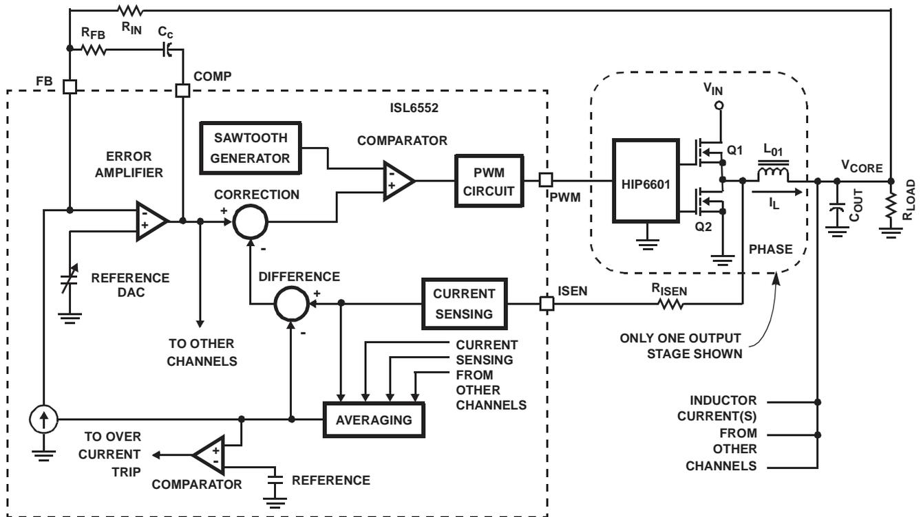
FIGURE 7. SIMPLIFIED FUNCTIONAL BLOCK DIAGRAM SHOWING CURRENT AND VOLTAGE SAMPLING
