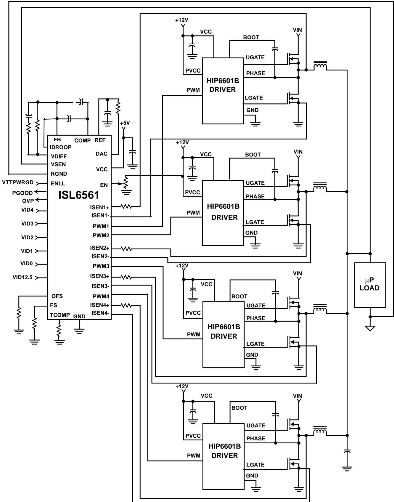
Typical Application - 4-Phase Buck Converter with DCR Sensing and Internal PTC
