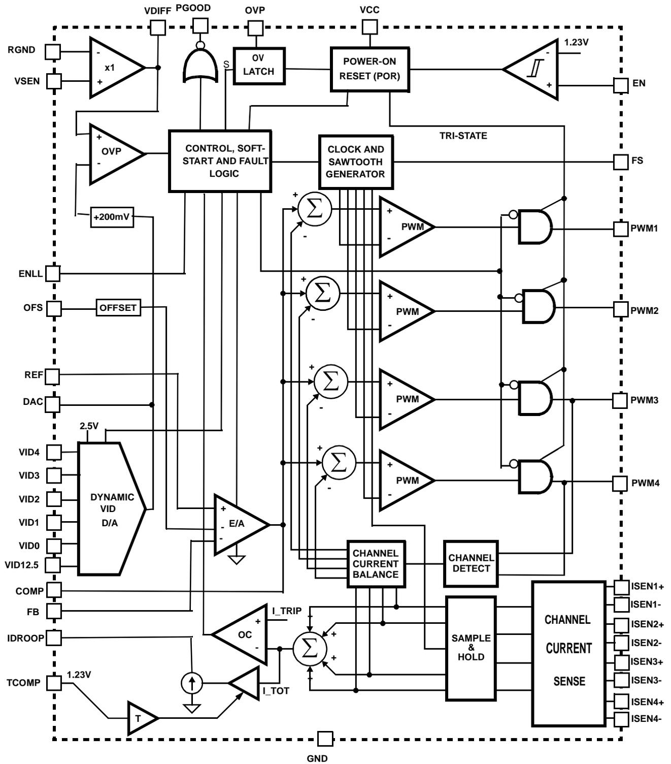
Typical Application - 4-Phase Buck Converter with  $R_{ds}$ , On Sensing and External NTC
