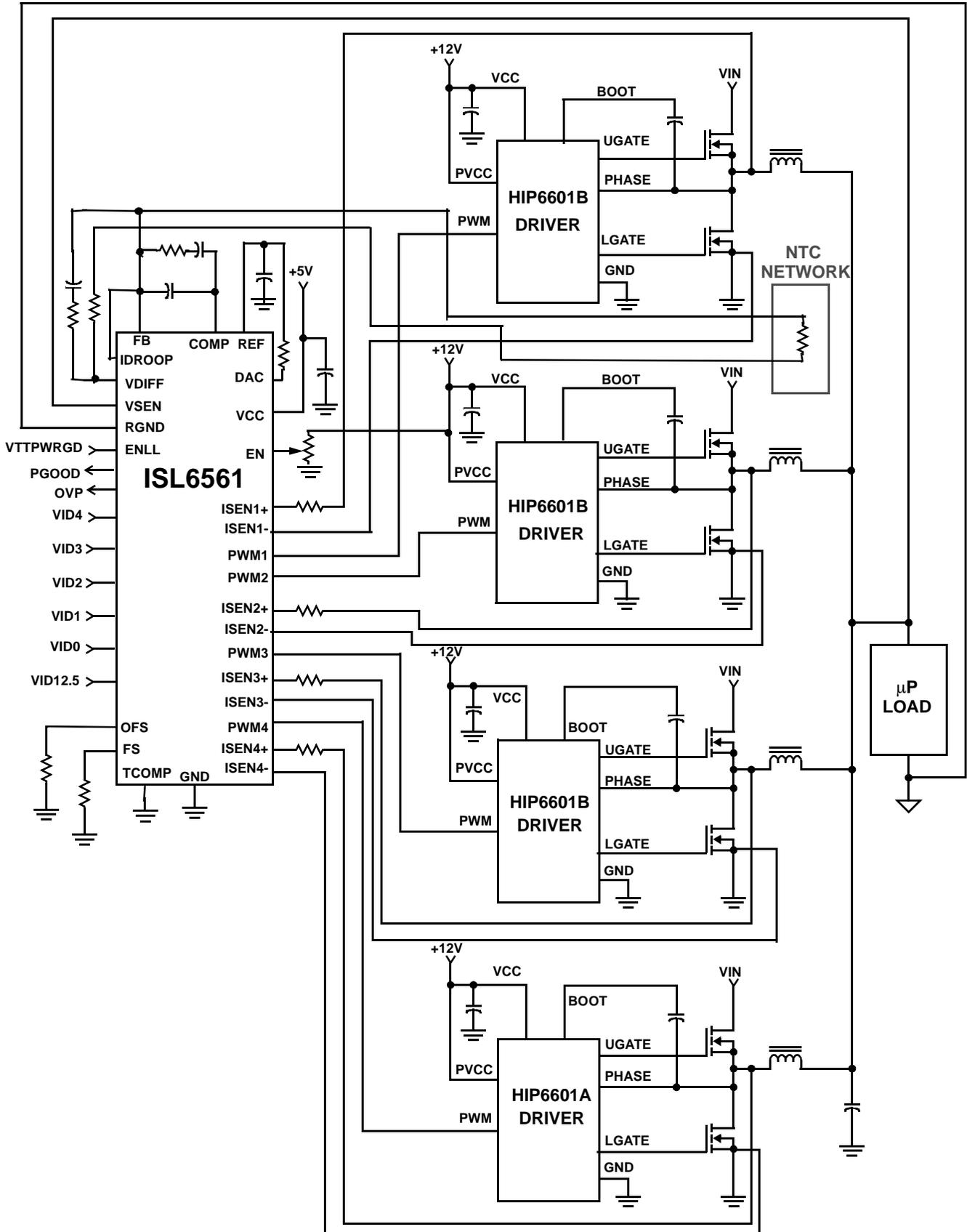
Typical Application - 4-Phase Buck Converter with Rdes, On Sensing and Internal PTC
