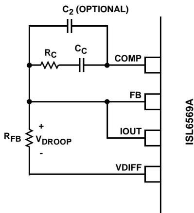
FIGURE 13. COMPENSATION CONFIGURATION FOR LOAD-LINE REGULATED ISL6569A CIRCUIT
