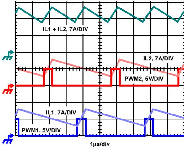
**FIGURE 2. PWM AND INDUCTOR-CURRENT WAVEFORMS FOR 2-PHASE CONVERTER**
