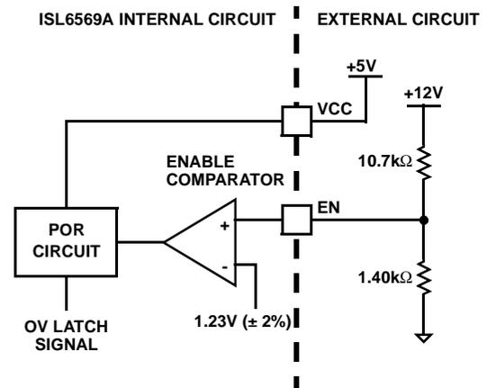
FIGURE 8. POWER SEQUENCING USING THRESHOLD-SENSITIVE ENABLE (EN) FUNCTION
