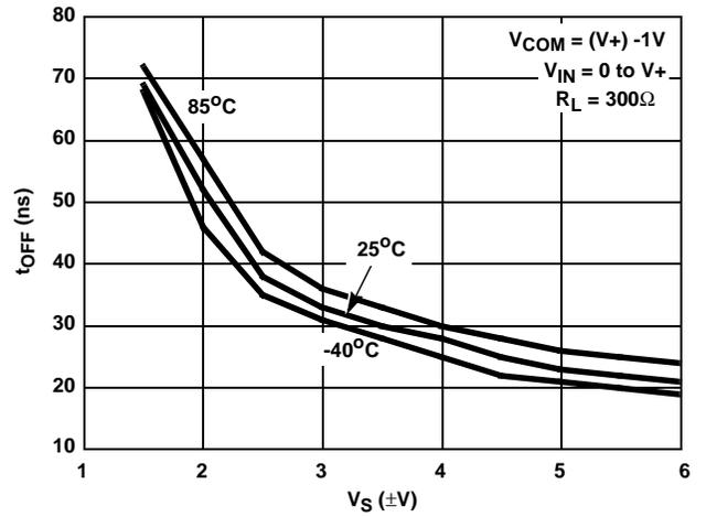
FIGURE 10. TURN - OFF TIME vs SUPPLY VOLTAGE
