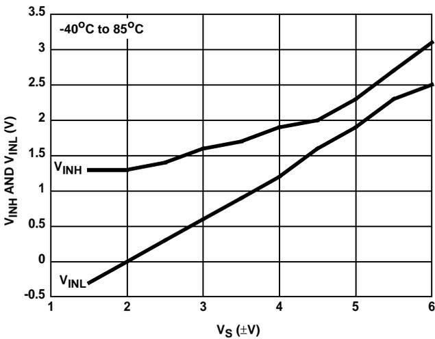
FIGURE 11. DIGITAL SWITCHING POINT vs SUPPLY VOLTAGE
