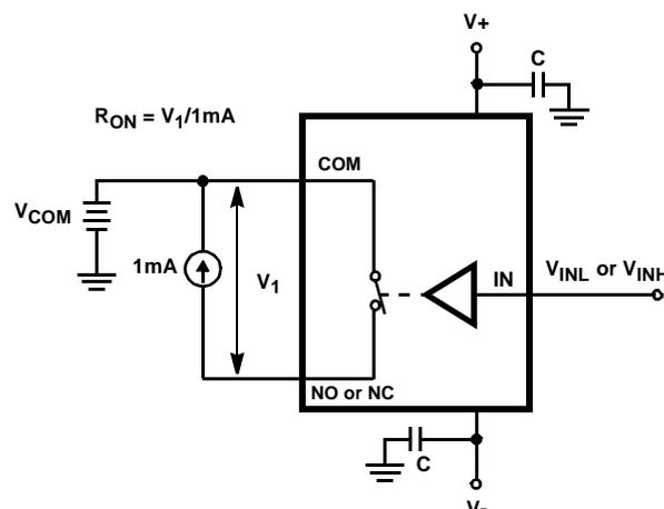
FIGURE 4.  $R_{ON}$  TEST CIRCUIT
