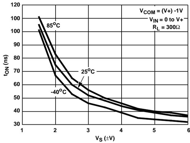
FIGURE 9. TURN - ON TIME vs SUPPLY VOLTAGE
