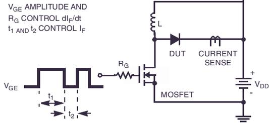
**Figure 12.  $I_{t_{rr}}$  Test Circuit**
