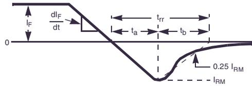
**Figure 13.  $t_{rr}$  Waveforms and Definitions**
