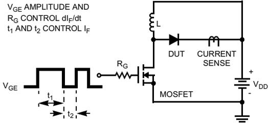
Figure 12.  $t_{rr}$  Test Circuit
