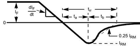
Figure 13.  $t_{rr}$  Waveforms and Definitions
