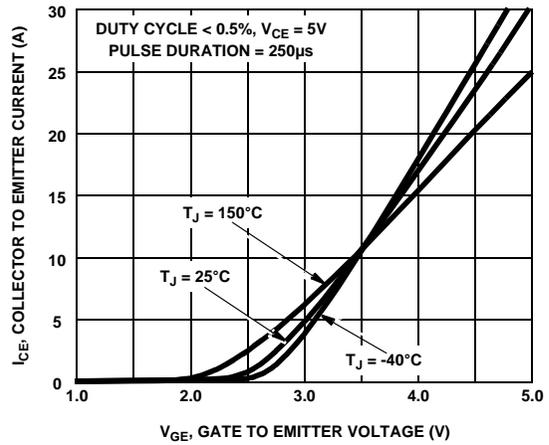
Figure 8. Transfer Characteristics
