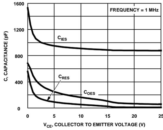
Figure 13. Capacitance vs Collector to Emitter Voltage
