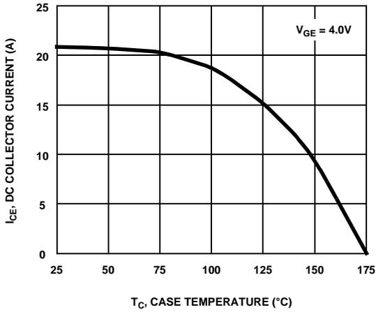
Figure 9. DC Collector Current vs Case Temperature
