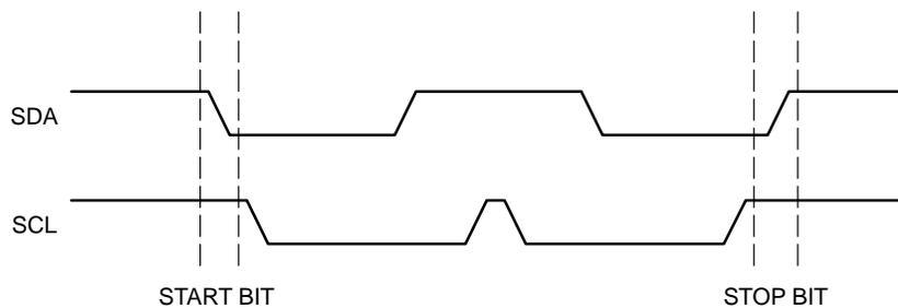
Figure 3. Start/Stop Timing
