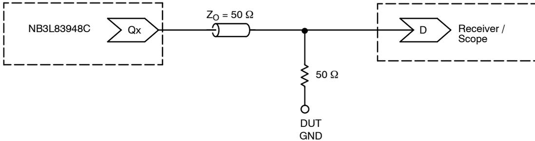
Figure 5. Typical Termination for Output Driver and Device Evaluation. Supplies may be centered on GND ( $\pm 1.65$  V or  $\pm 1.25$  V) to permit direct connection into 50  $\Omega$  to GND Scope modules
