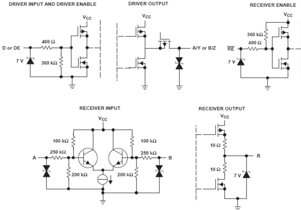
Figure 15. Equivalent Input and Output Schematic Diagrams
