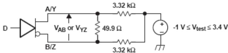
A. All resistors are 1% tolerance.
