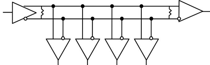
Figure 21. Multidrop or Distributed Simplex with Double Termination
