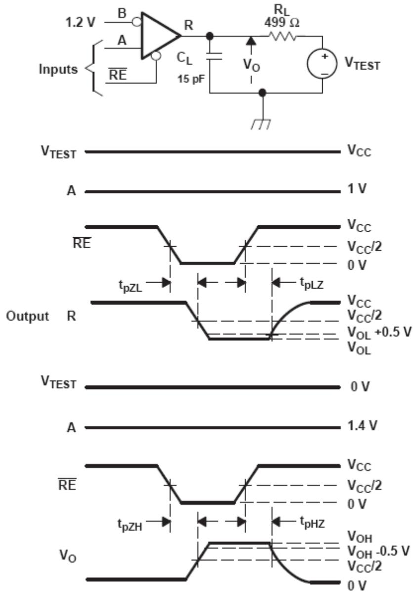
A. All input pulses are supplied by a generator having the following characteristics:  $t_r$  or  $t_f \leq 1$  ns, frequency = 500 kHz, duty cycle = 50  $\pm$ 5%.
