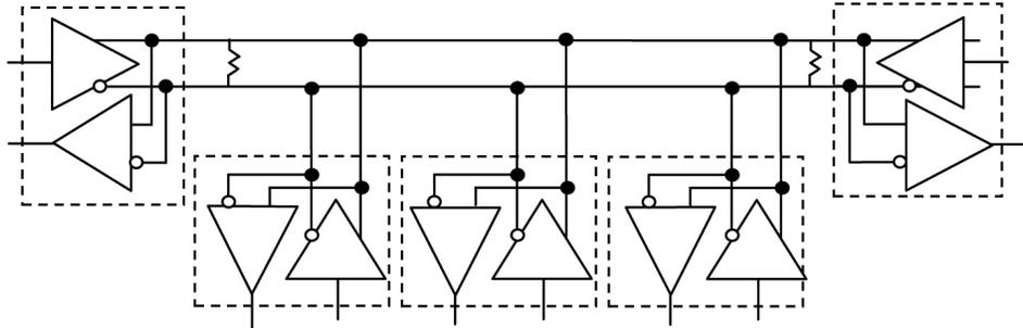
Figure 22. Multinode Multipoint Half Duplex (requires Double Termination)
