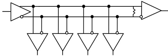
Figure 20. Multidrop or Distributed Simplex with Single Termination
