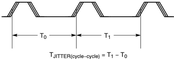
**Figure 8. Cycle-to-Cycle Jitter**
