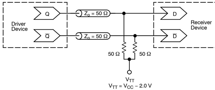
**Figure 10. Typical Termination for Output Driver and Device Evaluation
