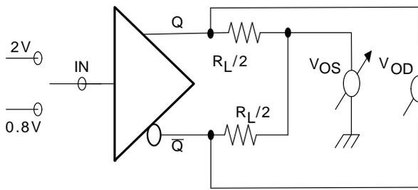
Figure 1. DC Test Circuit for Differential Driver
