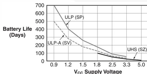
TinyLogic ULP and ULP-A with up to 50% less power consumption can extend your battery life significantly.
