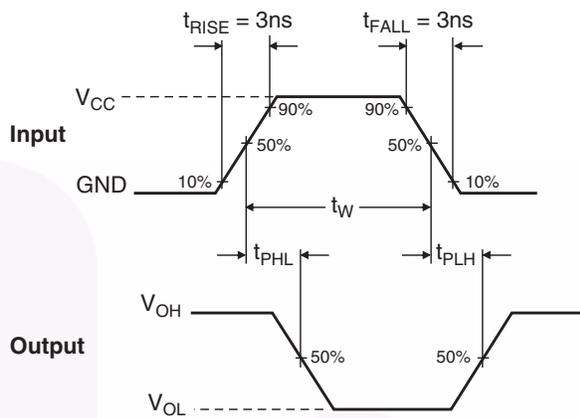
Figure 2. AC Waveforms
