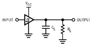
C<sub>L</sub> includes load and stray capacitance
