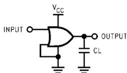
C<sub>L</sub> includes load and stray capacitance
