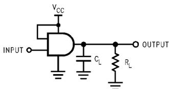
C<sub>L</sub> includes load and stray capacitance
