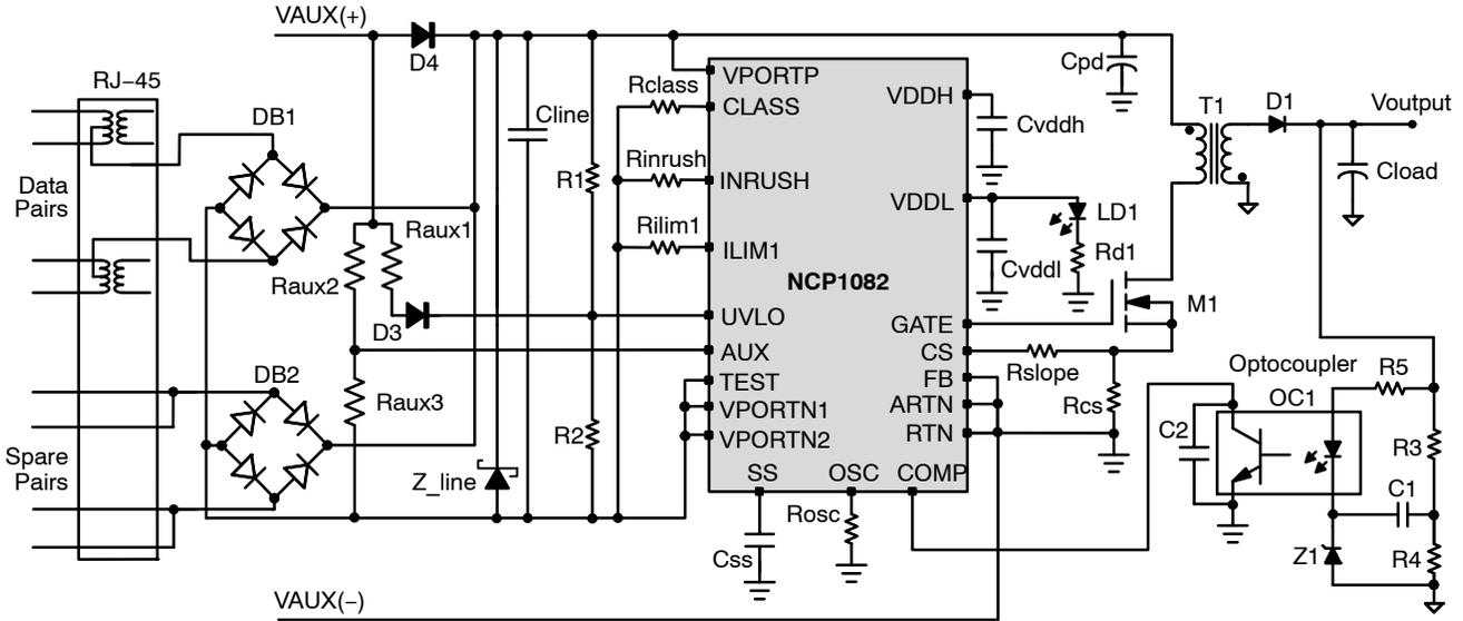
**Figure 2. Isolated Fly-back Converter with Rear Auxiliary Support**
