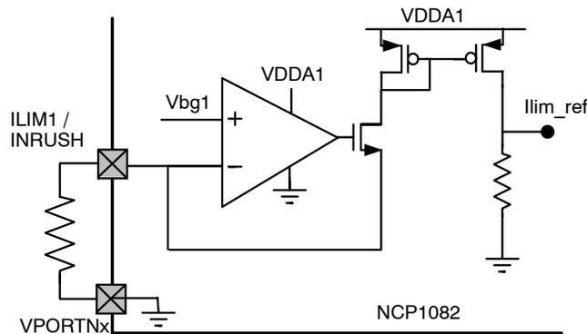
**Figure 12. Current Limitation Configuration (Inrush & Ilim1 Pins)**
