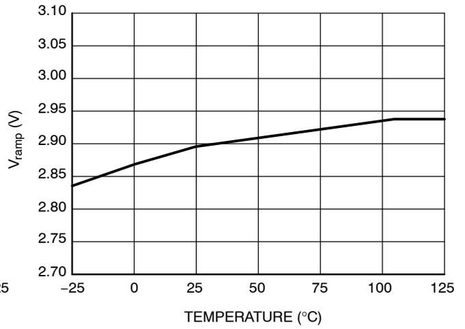
Figure 16. V<sub>ramp</sub> vs. Temperature
