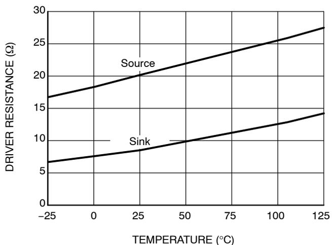
Figure 11. Drive Sink and Source Resistance vs. Temperature
