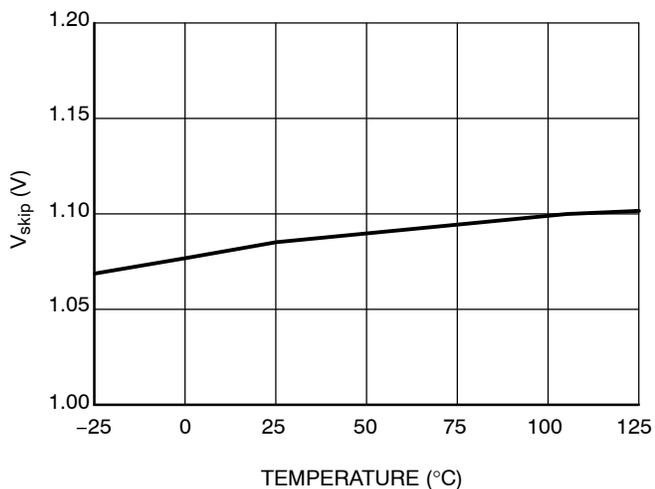
Figure 13. V<sub>skip</sub> vs. Temperature
