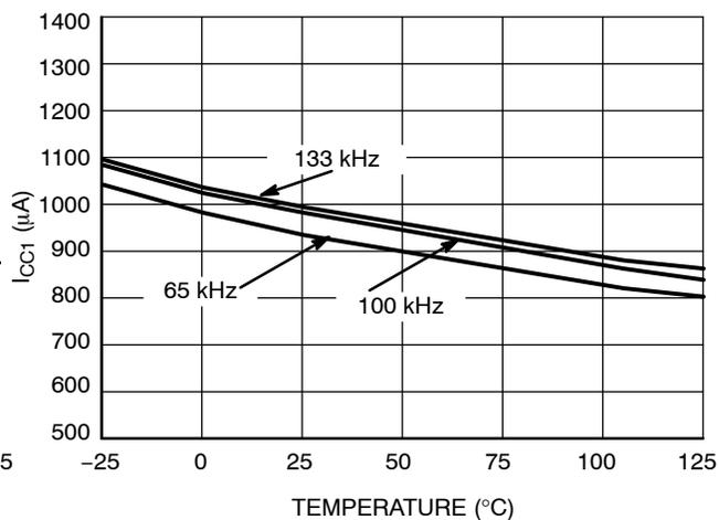
Figure 6. ICC1 (@ VCC = 11 V) vs. Temperature
