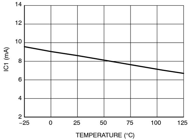
Figure 17. High Voltage Current Source (@ V<sub>CC</sub> = 10 V) vs. Temperature
