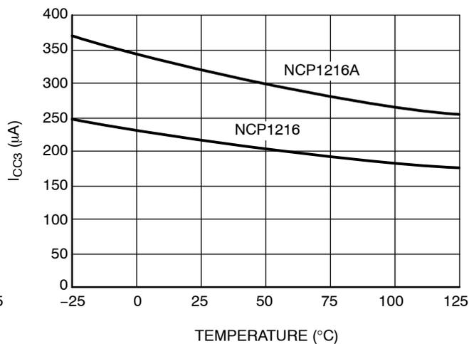
Figure 10. I<sub>CC3</sub> vs. Temperature
