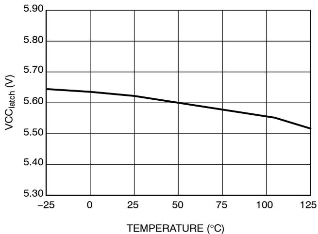
Figure 9. VCC<sub>latch</sub> vs. Temperature
