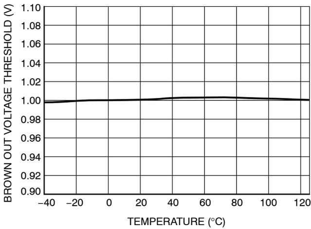
Figure 25. Brown Out Voltage Threshold vs. Junction Temperature
