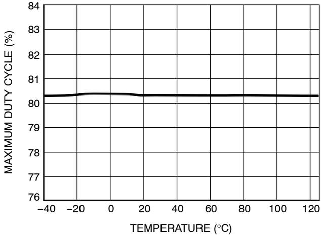
Figure 17. Maximum Duty-cycle, B Version vs. Junction Temperature
