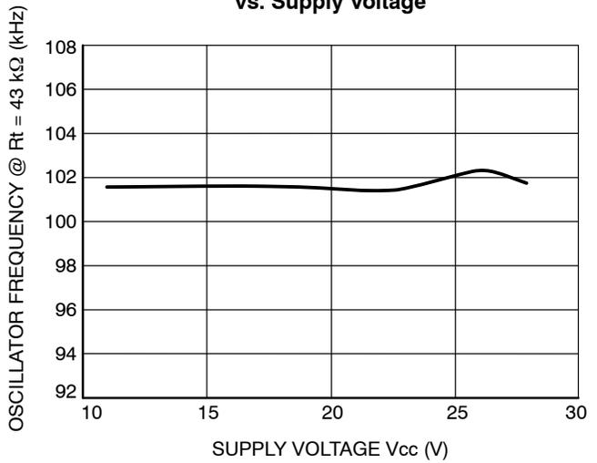
**Figure 14. Oscillator Frequency vs. Supply Voltage**
