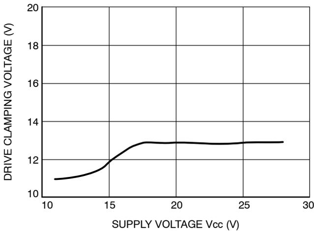
Figure 21. Drive Clamping Voltage vs. Supply Voltage
