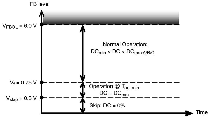
Figure 29. Mode of Operation versus the FB Pin Level
