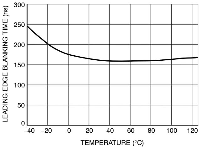
Figure 9. Leading Edge Blanking Time vs. Junction Temperature
