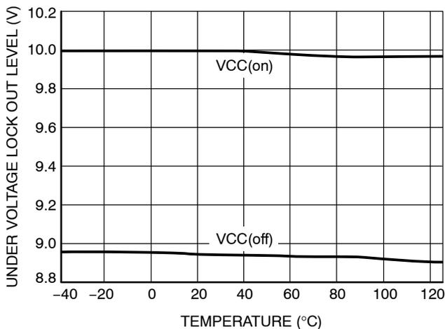
**Figure 3. Supply Voltage Threshold vs. Junction Temperature**
