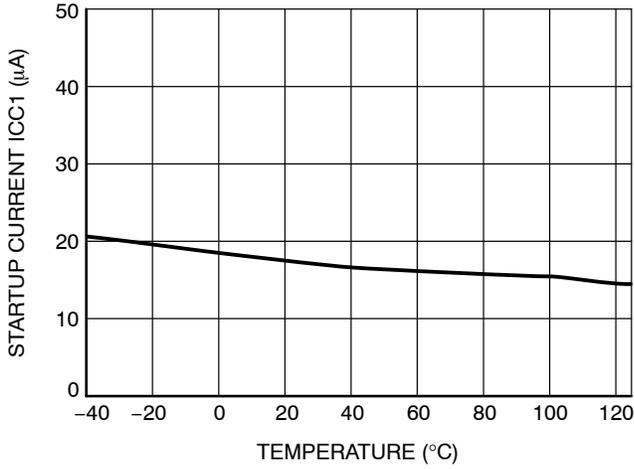
Figure 5. Start-up Current (I<sub>CC1</sub>) vs. Junction Temperature
