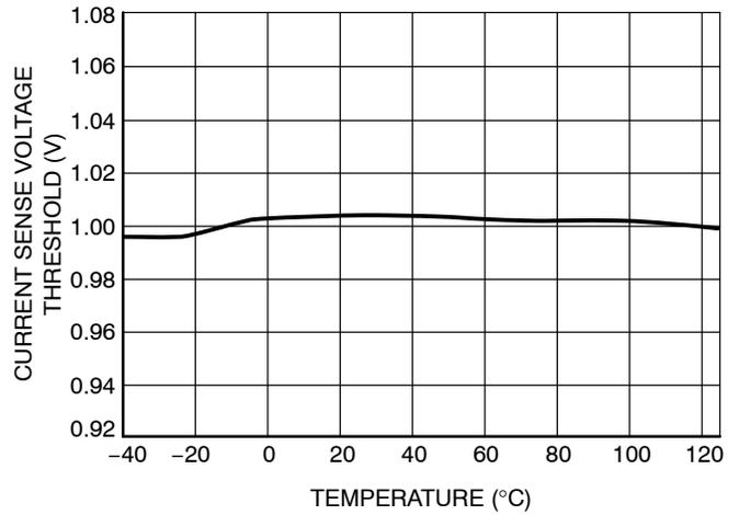
Figure 8. Current Sense Voltage Threshold vs. Junction Temperature
