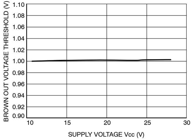
Figure 26. Brown Out Voltage Threshold vs. Supply Voltage
