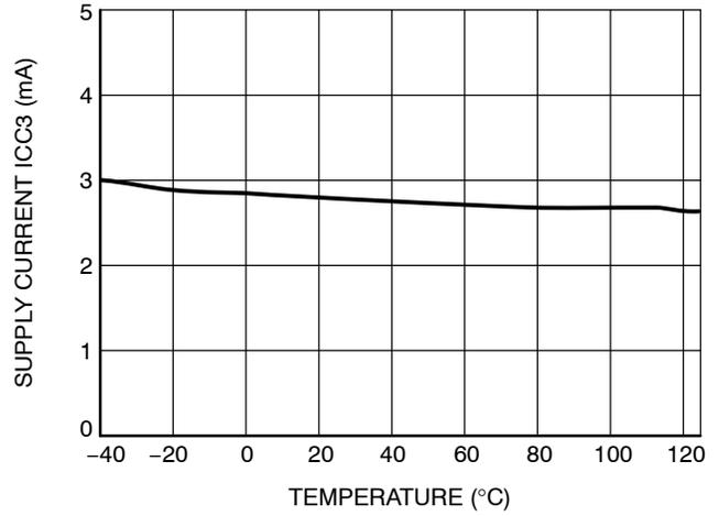
Figure 6. Supply Current (I<sub>CC3</sub>) vs. Junction Temperature
