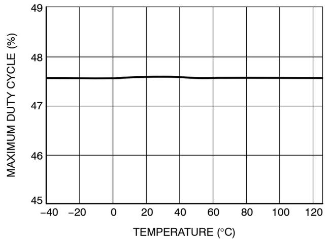
**Figure 16. Maximum Duty-cycle, A Version vs. Junction Temperature**
