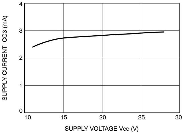
Figure 7. Supply Current (I<sub>CC3</sub>) vs. Supply Voltage
