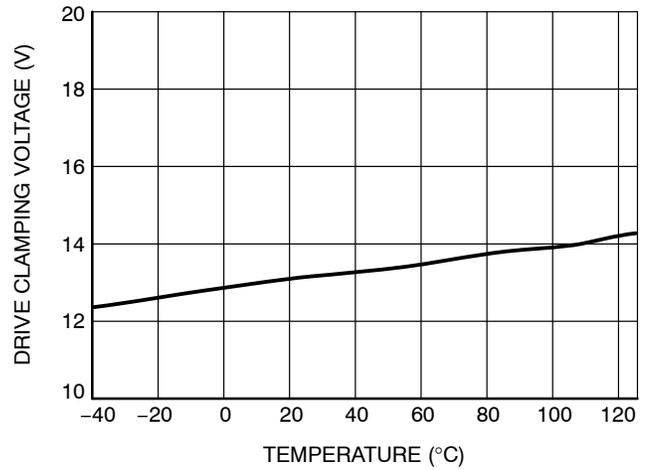
Figure 20. Drive Clamping Voltage vs. Junction Temperature
