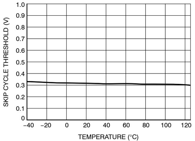
Figure 22. Skip Cycle Threshold vs. Junction Temperature
