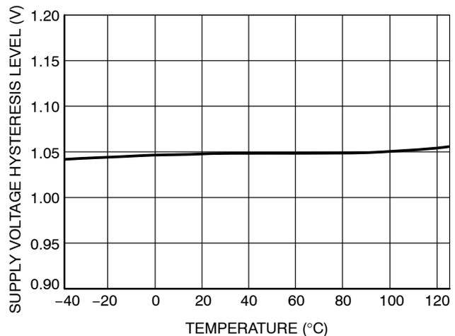
**Figure 4. Supply Voltage Hysteresis vs. Junction Temperature**
