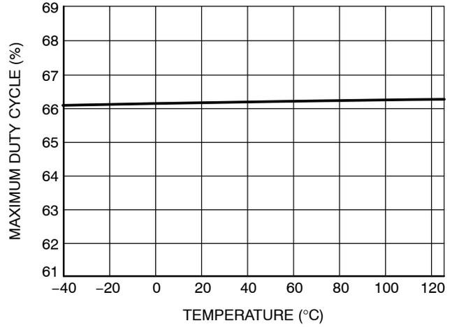
Figure 18. Maximum Duty-cycle, C Version vs. Junction Temperature
