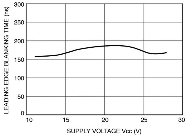
Figure 10. Leading Edge Blanking Time vs. Supply Voltage
