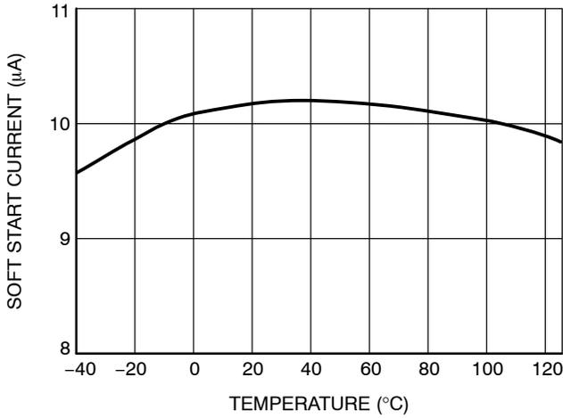
Figure 23. Soft Start Current vs. Junction Temperature
