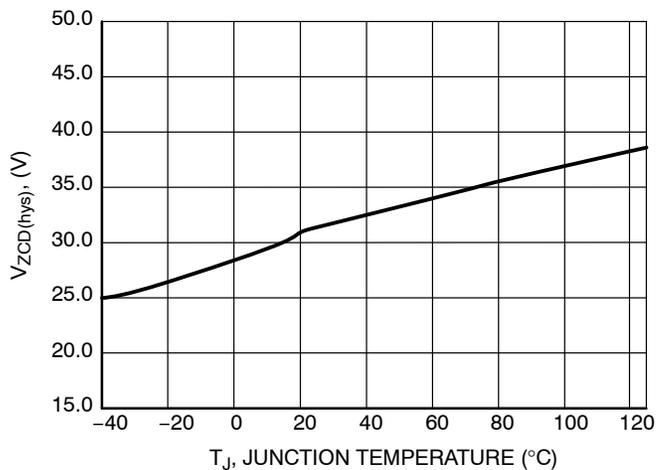
Figure 16.  $V_{ZCD(hys)}$  vs. Junction Temperature
