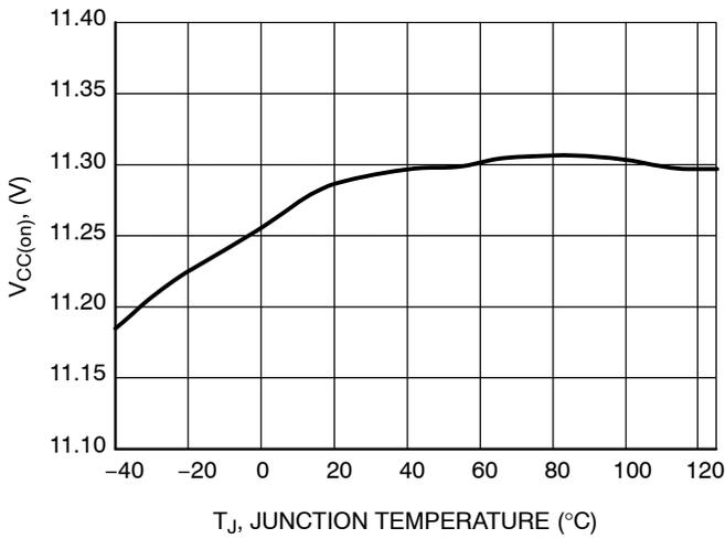
Figure 3.  $V_{CC(on)}$  vs. Junction Temperature
