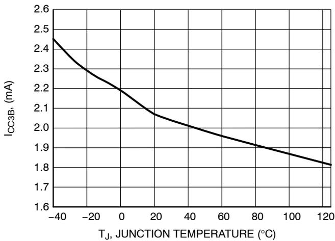
Figure 7.  $I_{CC3B}$  vs. Junction Temperature
