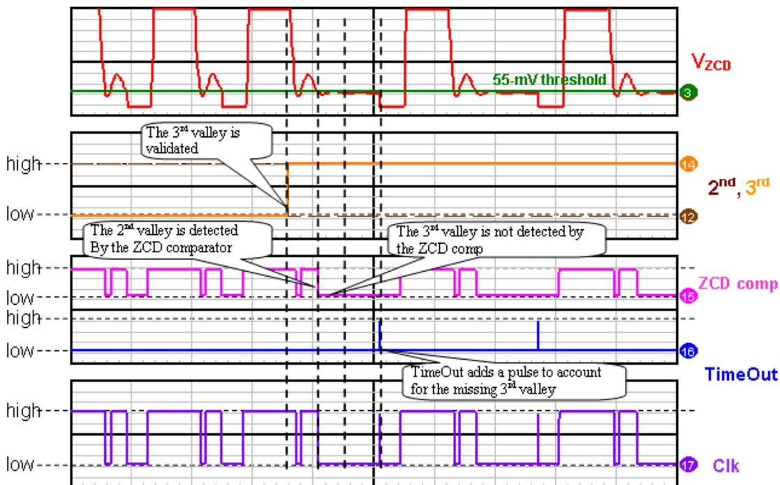
Figure 30. Time Out Case n°1: the 3<sup>rd</sup> Valley is Missing
