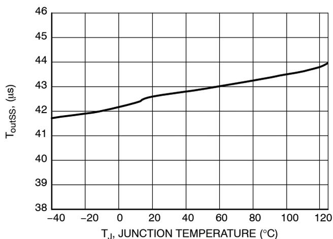
Figure 18.  $T_{outSS}$  vs. Junction Temperature
