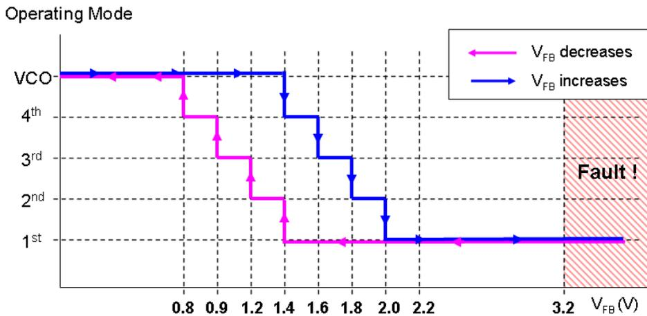
Figure 22. Operating Valley According to FB Voltage
