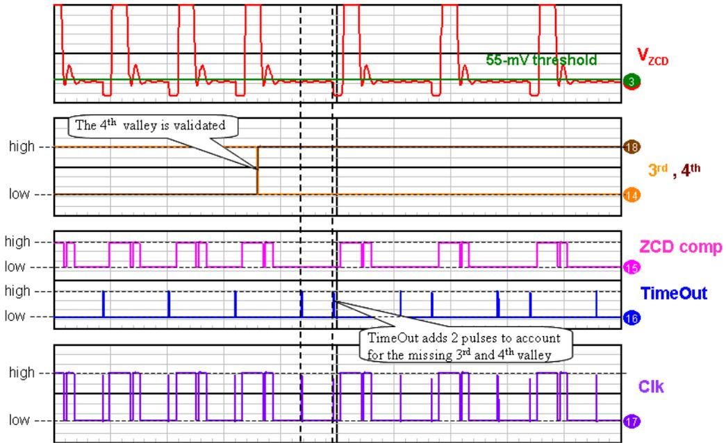
Figure 31. Time Out Case n°2: the 3<sup>rd</sup> and 4<sup>th</sup> Valley are Missing
