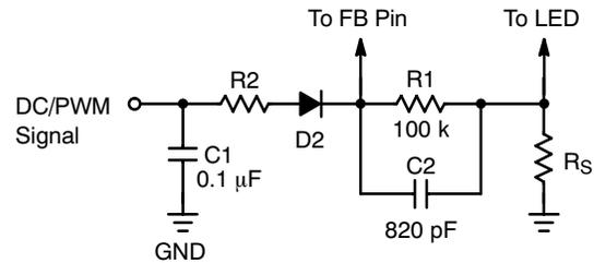
With this additional circuit, the maximum LED current is set by the above equation. The value of R<sub>2</sub> can be obtained by the following equation:
