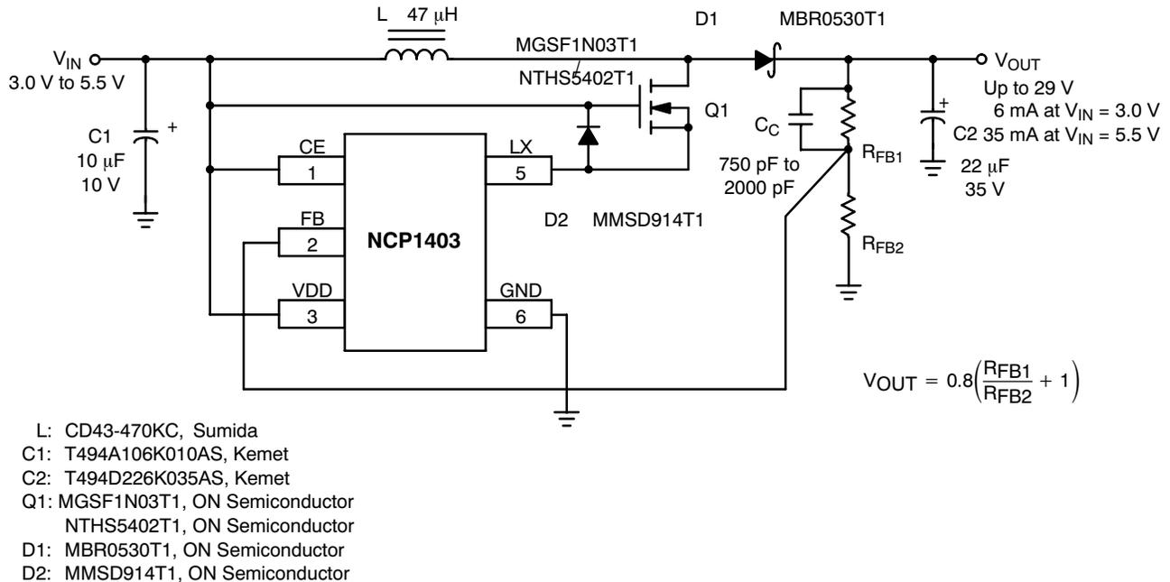
Figure 33. Step-Up DC-DC Converter with 29 V Output Voltage
