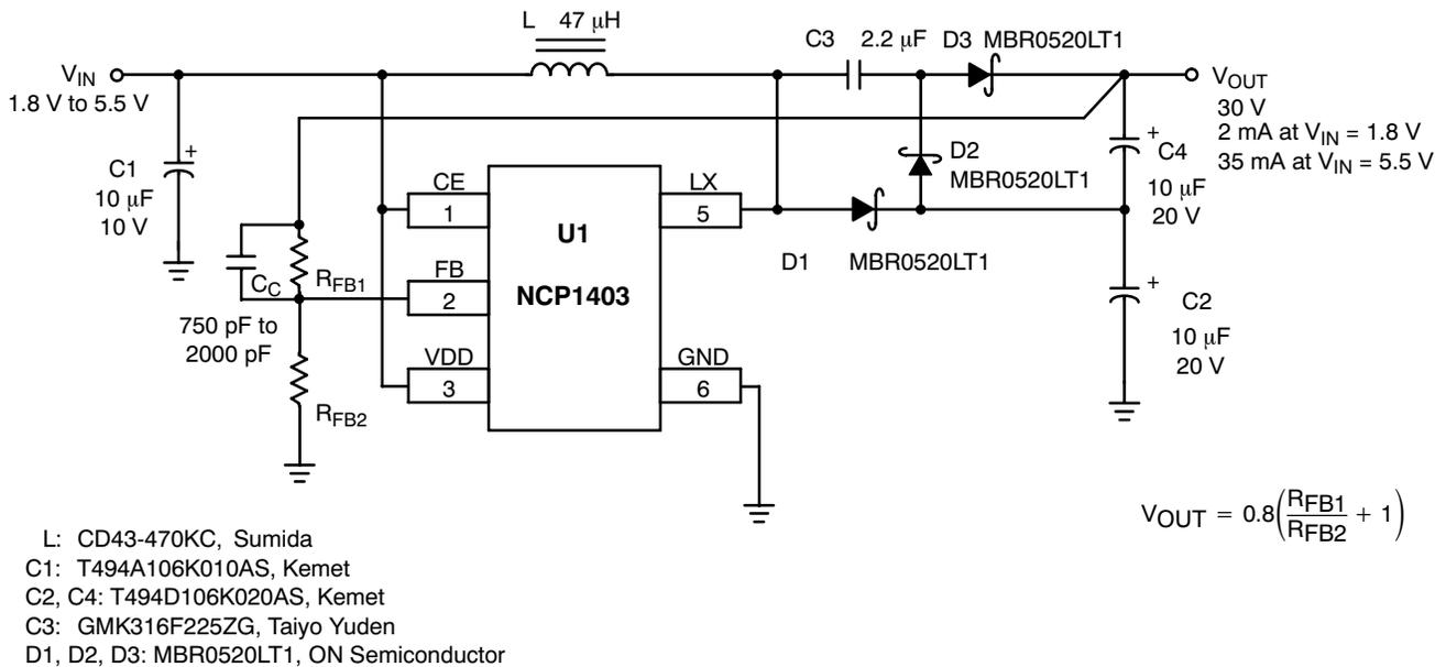
**Figure 35. Step-Up DC-DC Converter with 30 V Output Voltage**
