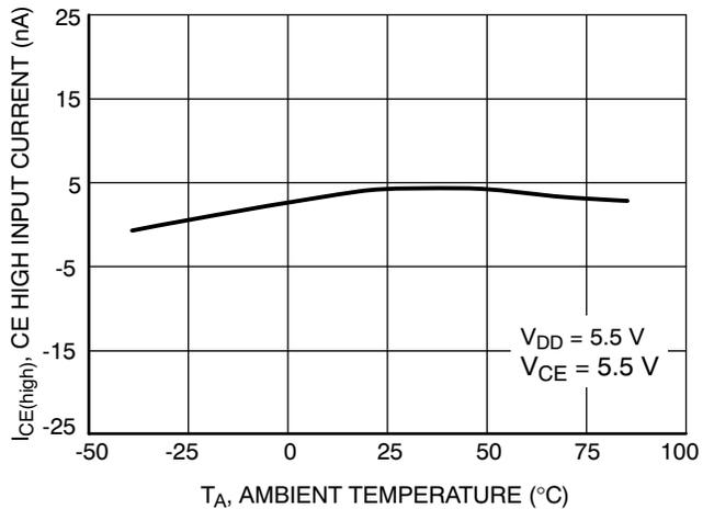
Figure 21. CE High Input Current versus Ambient Temperature
