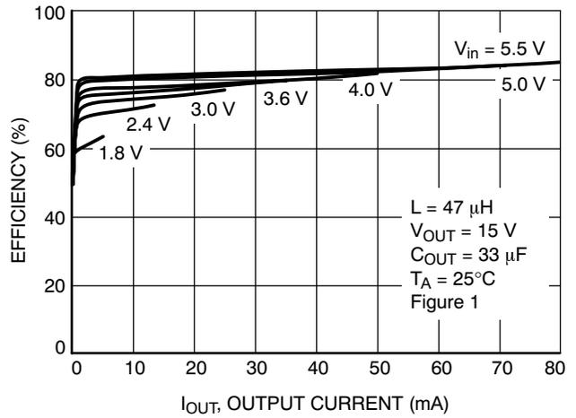
Figure 5. Efficiency versus Output Current ( $V_{OUT} = 15 \text{ V}$ )
