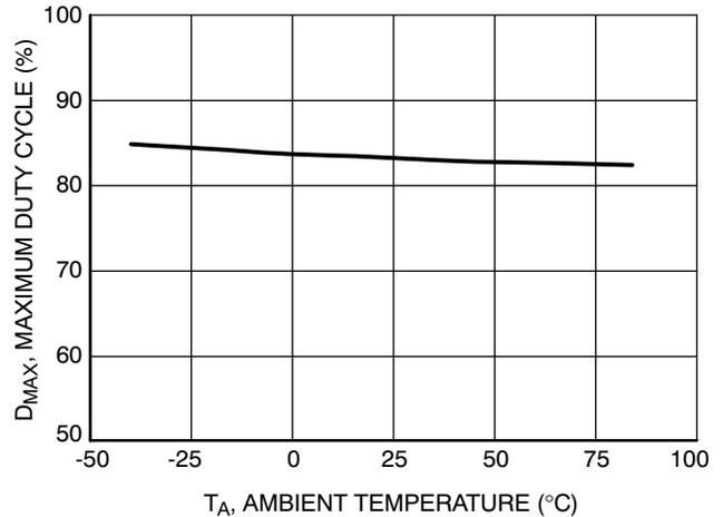
Figure 15. Maximum Duty Cycle versus Ambient Temperature
