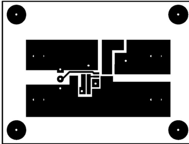
Figure 29. Step-Up Converter Demonstration Board Top Layer Copper
