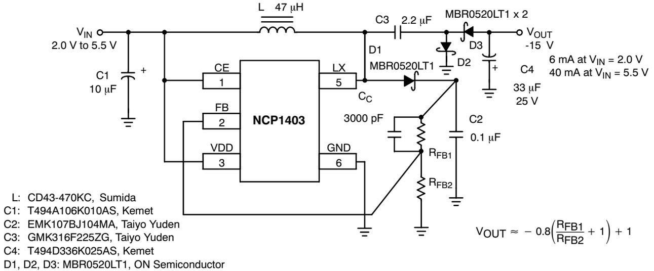
Figure 32. Positive-to-Negative Output Converter for Negative LCD Bias
