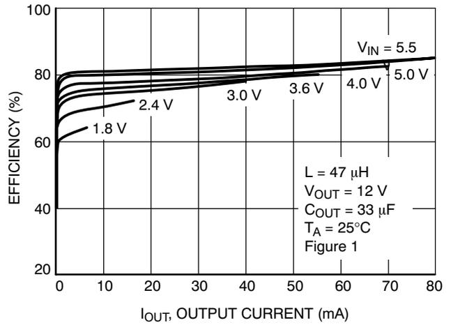
Figure 7. Efficiency versus Output Current ( $V_{OUT} = 12 \text{ V}$ )
