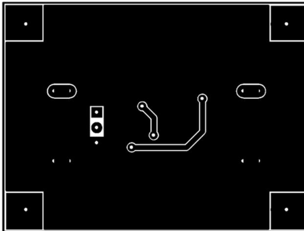
Figure 30. Step-Up Converter Demonstration Board Bottom Layer Copper
