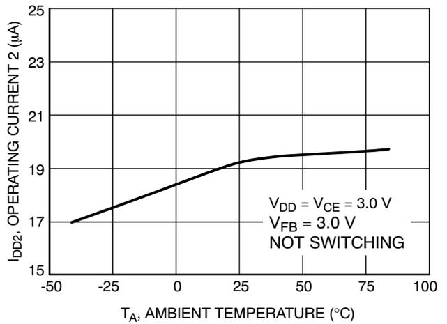
Figure 19. Operating Current 2 versus Ambient Temperature
