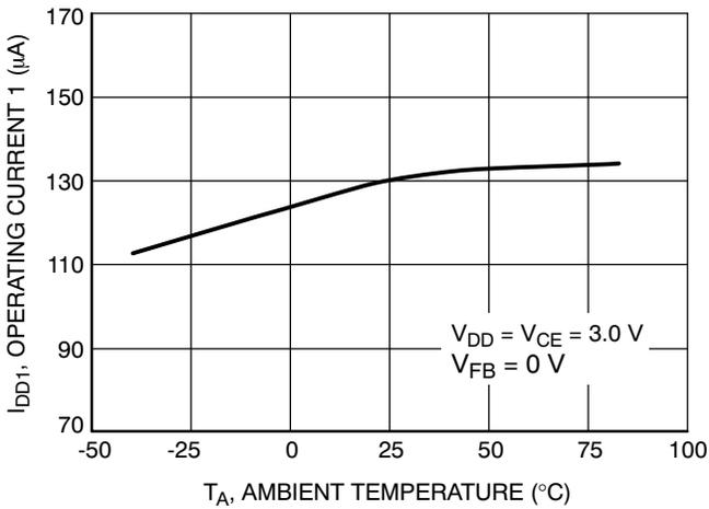
Figure 18. Operating Current 1 versus Ambient Temperature
