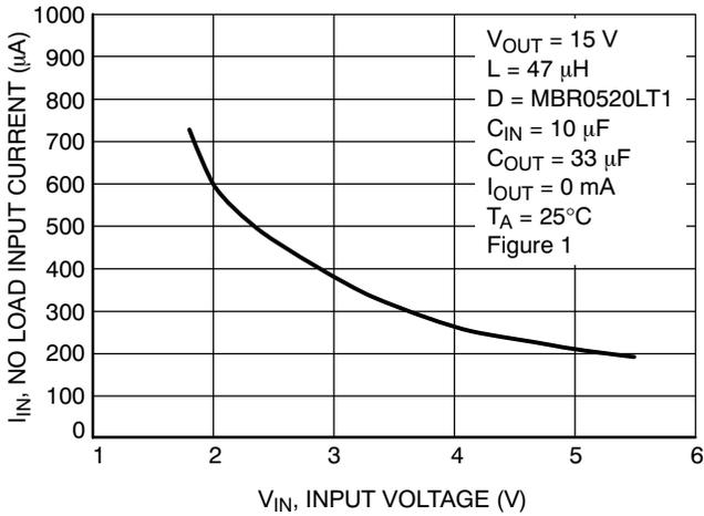
Figure 10. No Load Input Current versus Input Voltage
