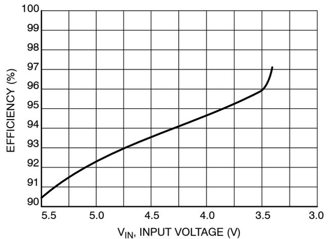
Figure 9. Maximum Efficiency vs. Input Voltage
