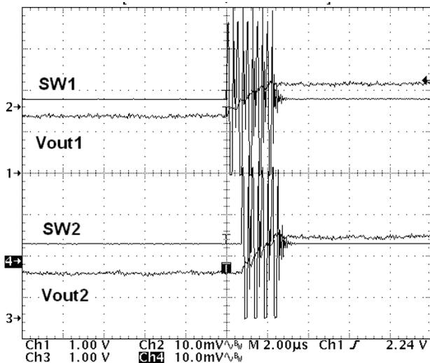
**Figure 23. PFM Switching Waveforms**
