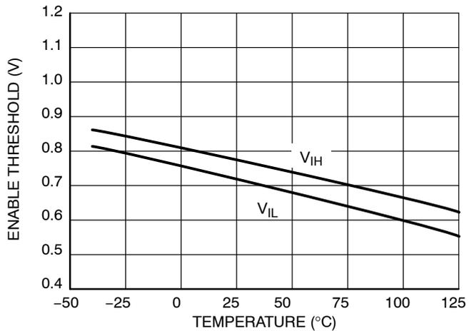
Figure 21. Enable Thresholds  $V_{IN} = 3.6 \text{ V}$ ,
