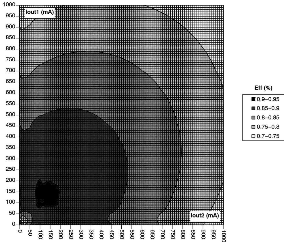
Figure 3. Efficiency vs. Output Current ( $V_{IN} = 3.6\text{ V}$ ,  $V_{OUT1} = 1.8\text{ V}$ ,  $V_{OUT2} = 1.8\text{ V}$ , Temperature =  $25^{\circ}\text{C}$ )
