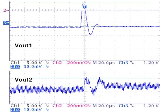
**Figure 15. Load Transient and Crosstalk,**
