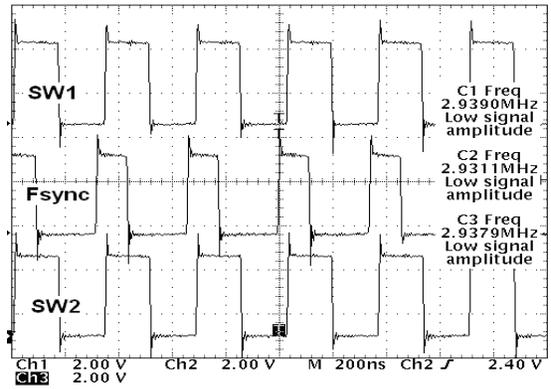
Figure 17. External Synchronization,  $F_{sync} = 2.93 \text{ MHz}$
