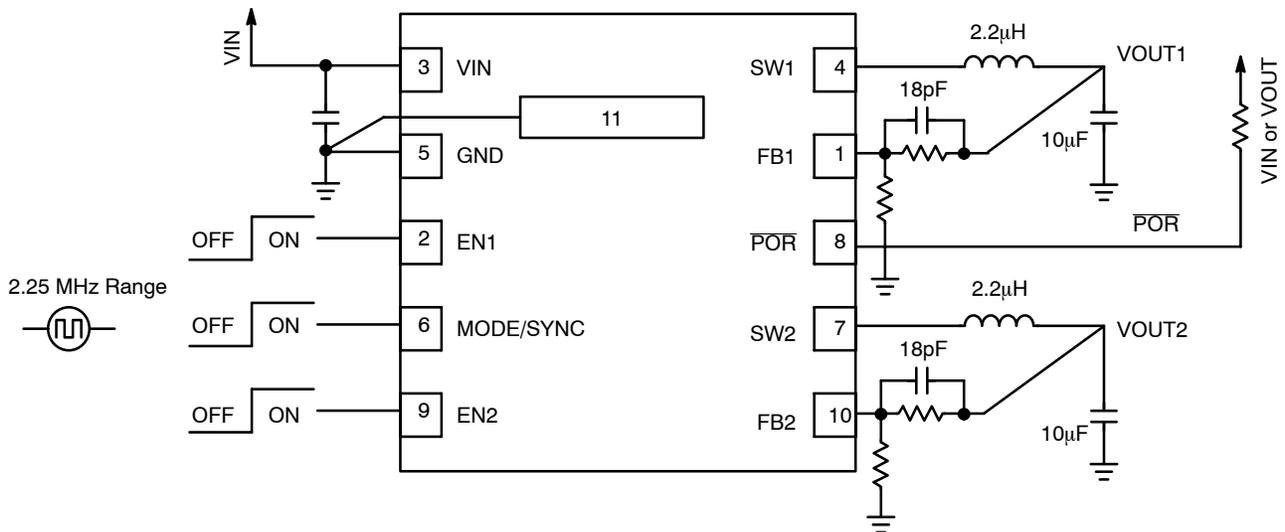
NOTE: Exposed pad of UDFN10 package – named pin11 – must be connected to system ground.
