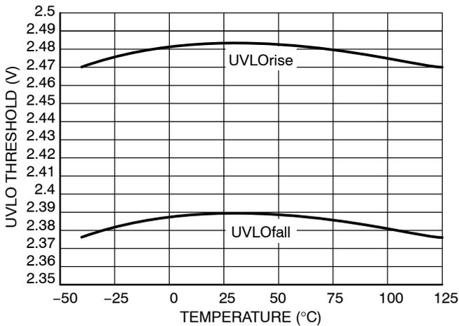
Figure 20. UVLO Thresholds  $V_{IN} = 3.6 \text{ V}$ ,
