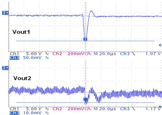
**Figure 14. Load Transient and Crosstalk,**
