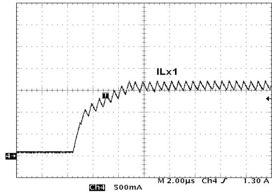
Figure 19. Current Peak Inductor Protection
