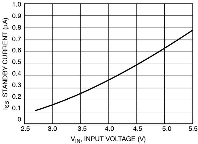
**Figure 10. Standby Current vs. Input Voltage**
