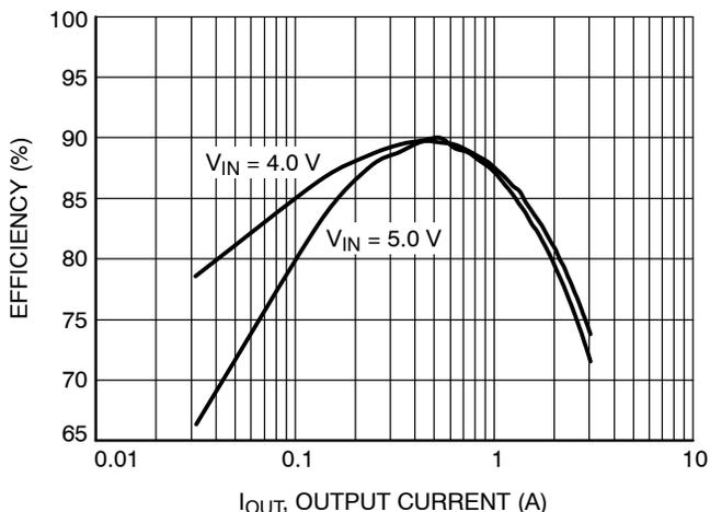
Figure 5. Efficiency vs. Output Current (1.05 V)
