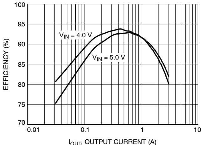
Figure 4. Efficiency vs. Output Current (1.8 V)
