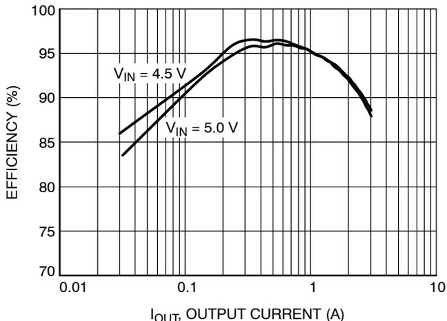
Figure 3. Efficiency vs. Output Current (3.3 V)
