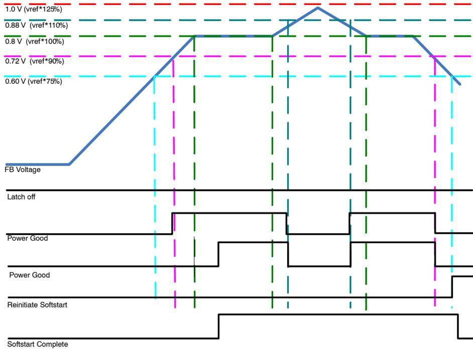
**Figure 35. Powerup Sequence and Undervoltage Soft-Start**
