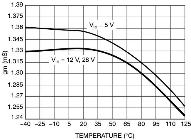
Figure 9. Transconductance vs. Input Voltage and Temperature
