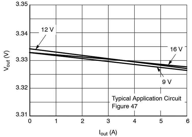
Figure 4. Load Regulation vs. Input Voltage
