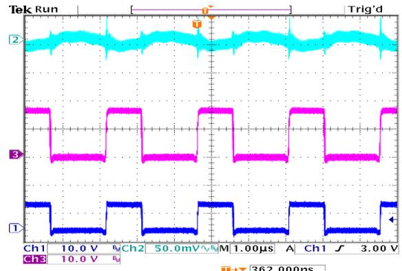
Input = 9 V, Output = 3.3 V, Load = 5 A
