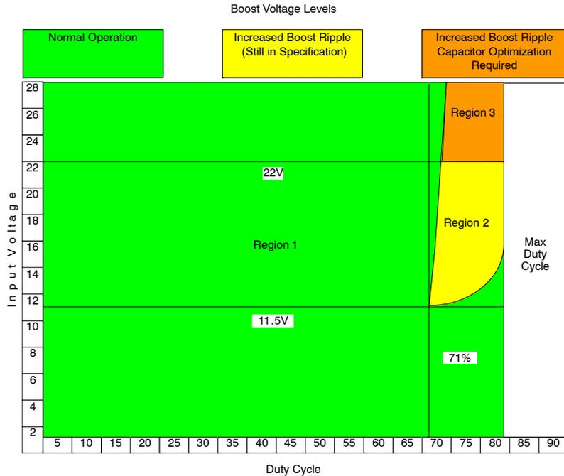
**Figure 39. Safe Operating Area for Boost Voltage with a 0.1  $\mu\text{F}$  Capacitor**
