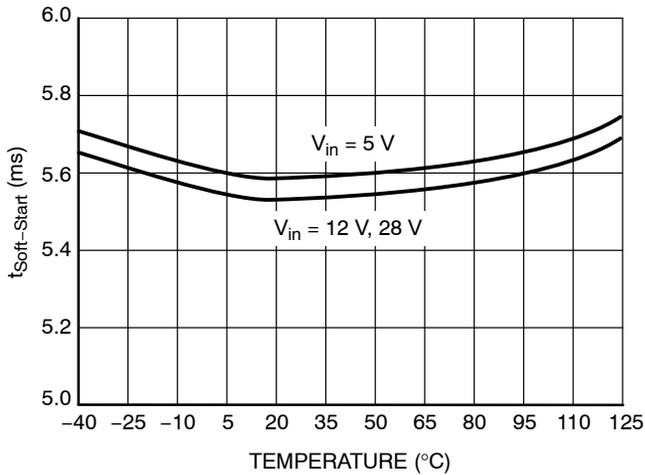
Figure 21. Soft-Start Time vs. Input Voltage and Temperature
