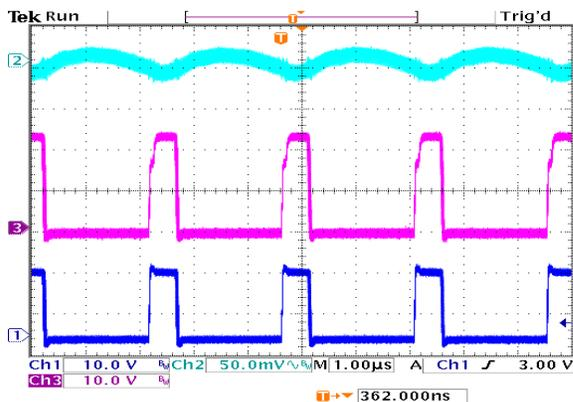
Input = 16 V, Output = 3.3 V, Load = 0 A
