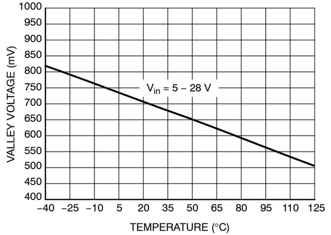
Figure 16. Valley Voltage vs. Input Voltage and Temperature
