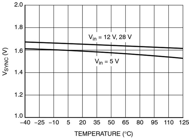
Figure 15. SYNC Threshold vs. Input Voltage and Temperature
