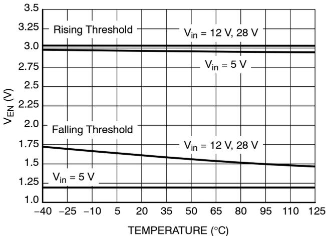
Figure 13. Enable Threshold vs. Input Voltage and Temperature
