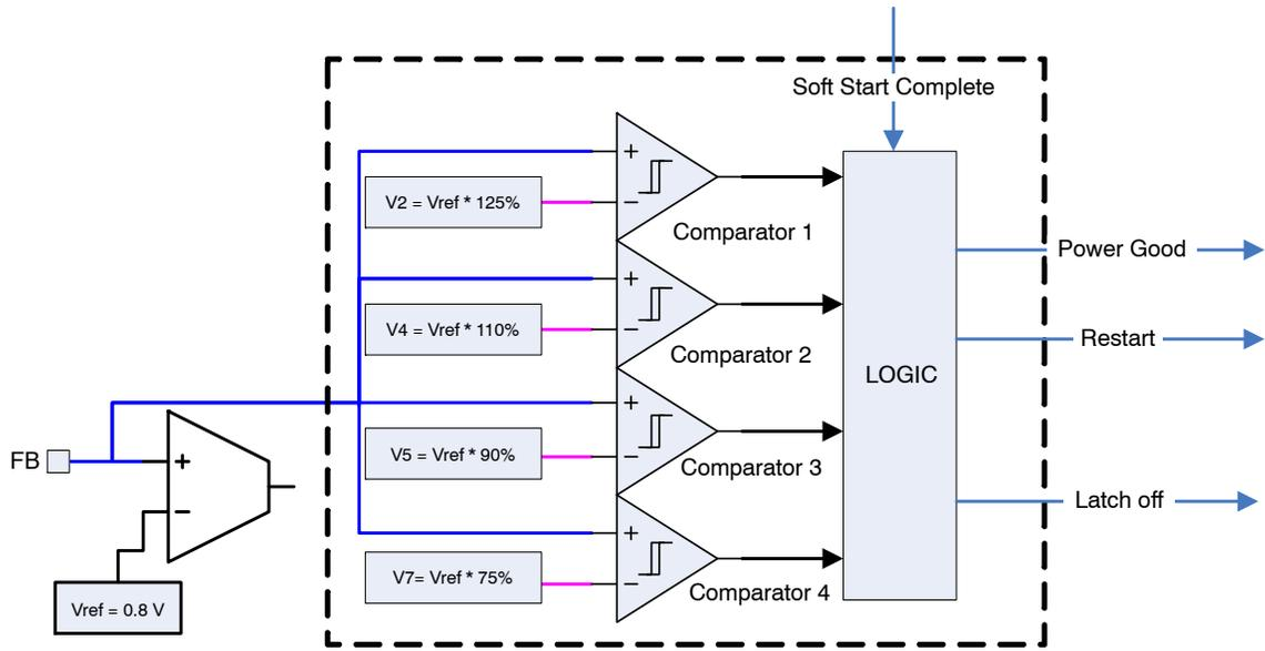
Figure 32. OOV, OUV, and Power Good Circuit Diagram
