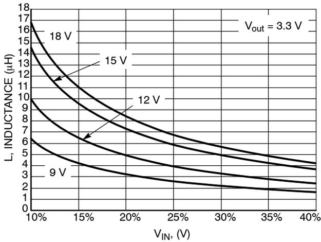
**Figure 42. Ripple Current Ratio vs. Inductance**
