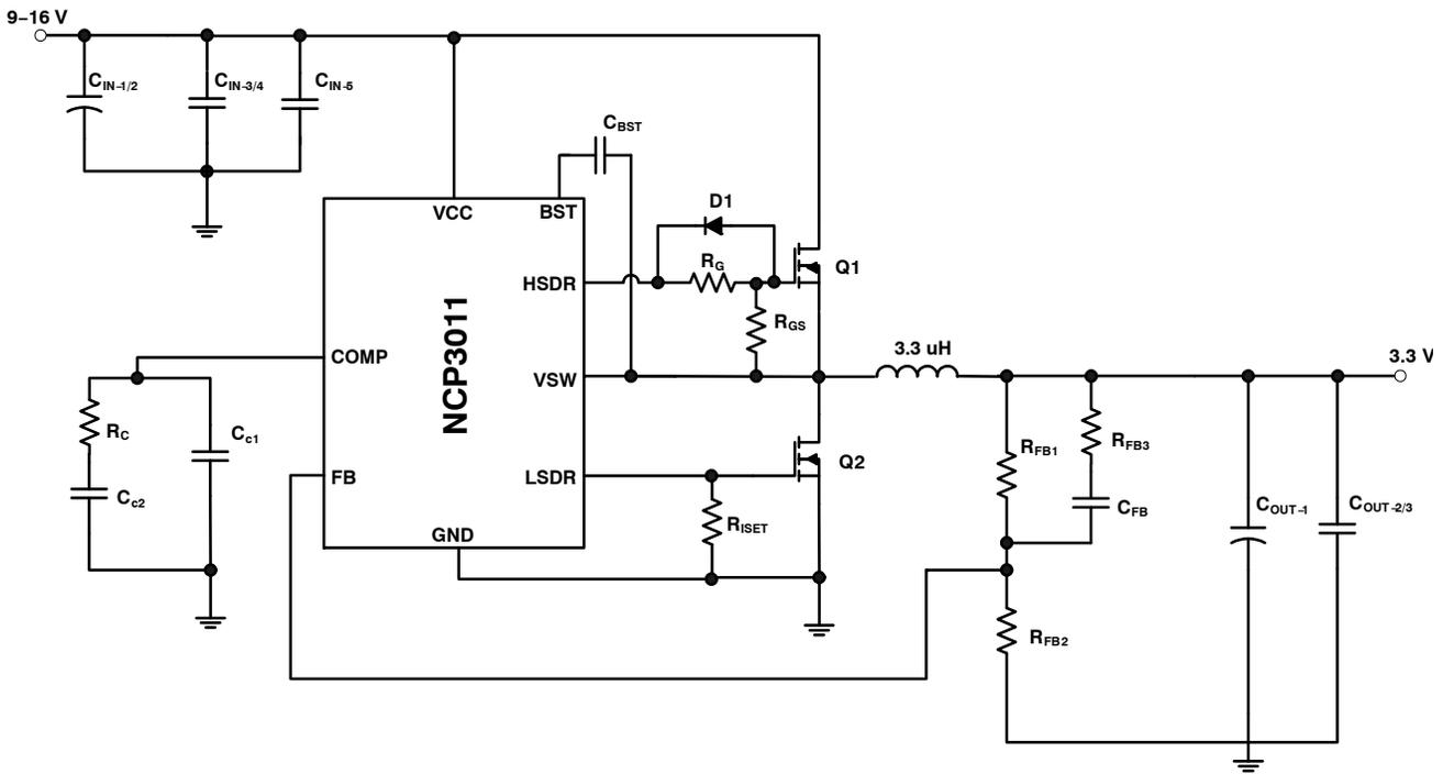
Figure 47. Typical Application,  $V_{IN} = 9 - 16 \text{ V}$ ,  $V_{OUT} = 3.3 \text{ V}$ ,  $I_{OUT} = 6 \text{ A}$
