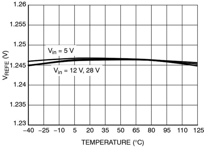
Figure 17. External Reference Voltage vs. Input Voltage and Temperature
