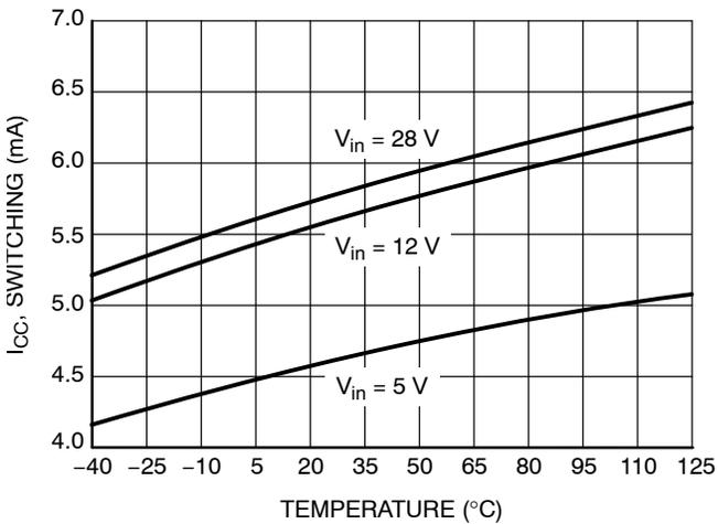
Figure 7. Supply Current vs. Input Voltage and Temperature
