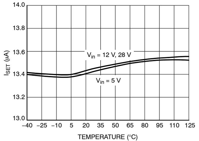
Figure 22. Current Limit Set Current vs. Temperature
