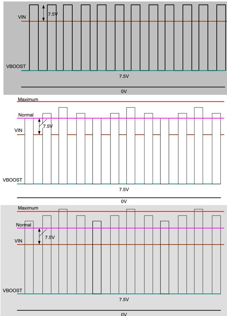
**Figure 40. Typical Waveforms for Region 1 (top), Region 2 (middle), and Region 3 (bottom)**
