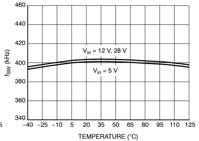
Figure 6. Switching Frequency vs. Input Voltage and Temperature
