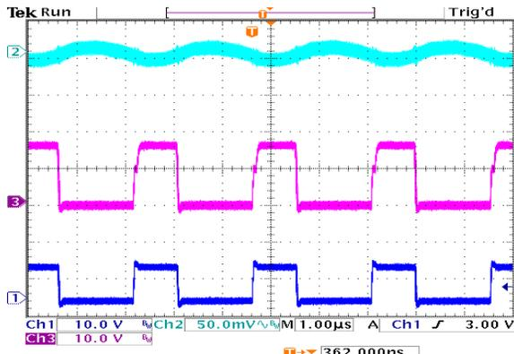
Input = 9 V, Output = 3.3 V, Load = 0 A
