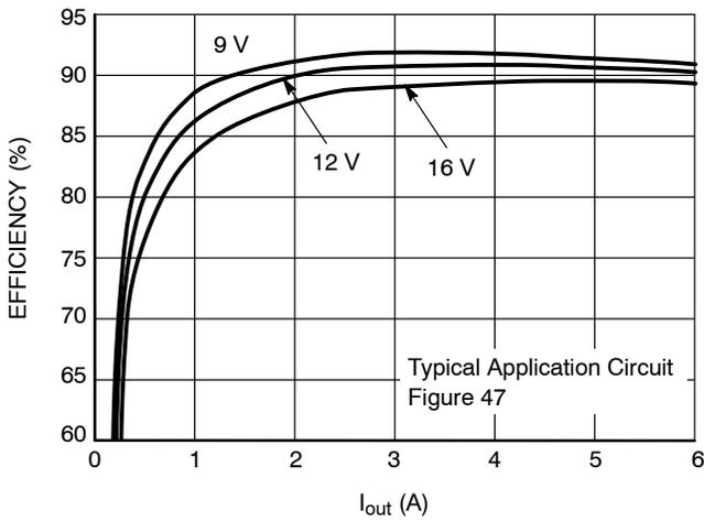
Figure 3. Efficiency vs. Output Current and Input Voltage
