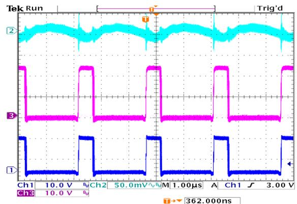
Input = 16 V, Output = 3.3 V, Load = 5 A
