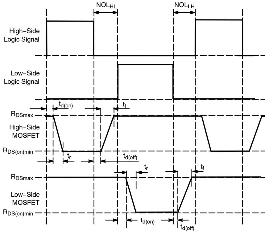
Figure 44. MOSFETs Timing Diagram
