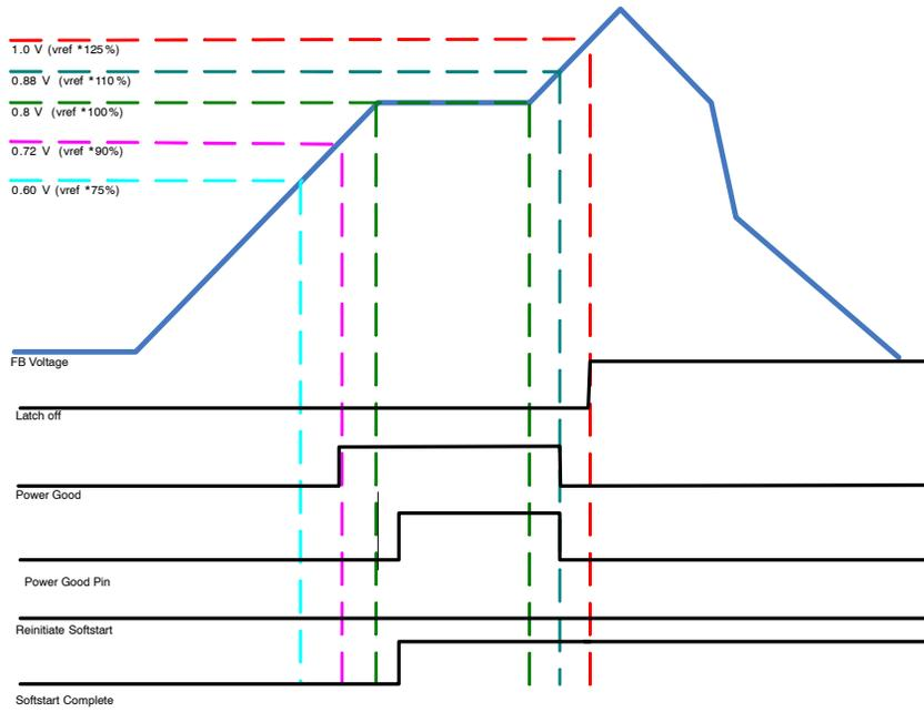
**Figure 34. Powerup Sequence and Overvoltage Latch**
