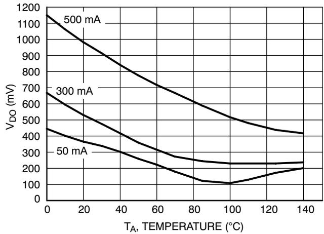
**Figure 14. Dropout Voltage vs. Temperature
