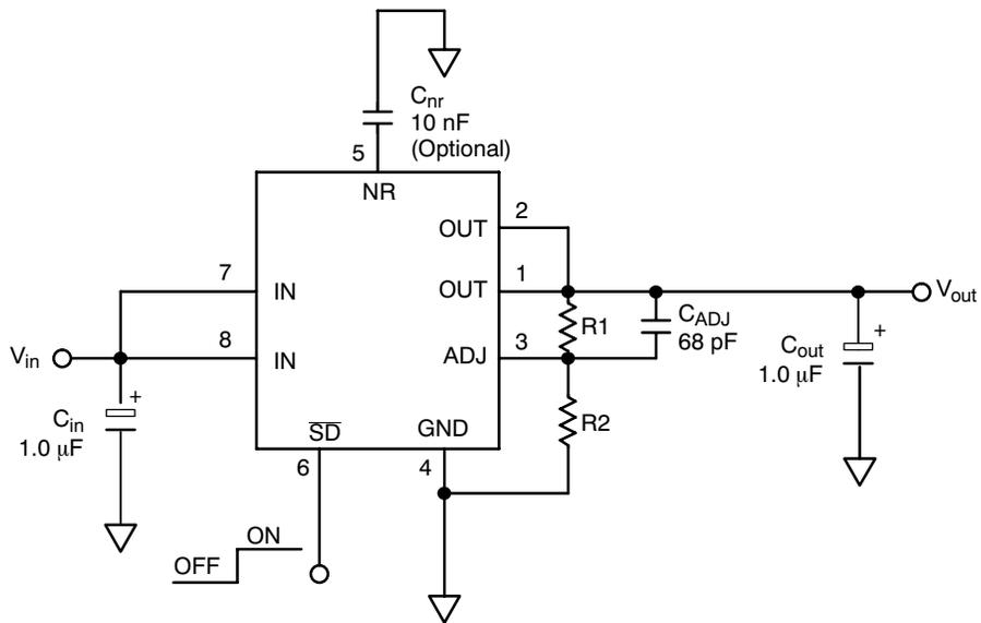
Figure 2. Typical Adjustable Version Application Schematic (Micro8 Package)
