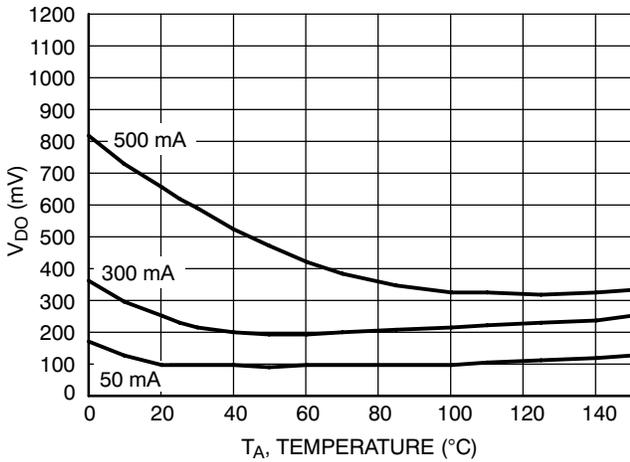
**Figure 13. Dropout Voltage vs. Temperature
