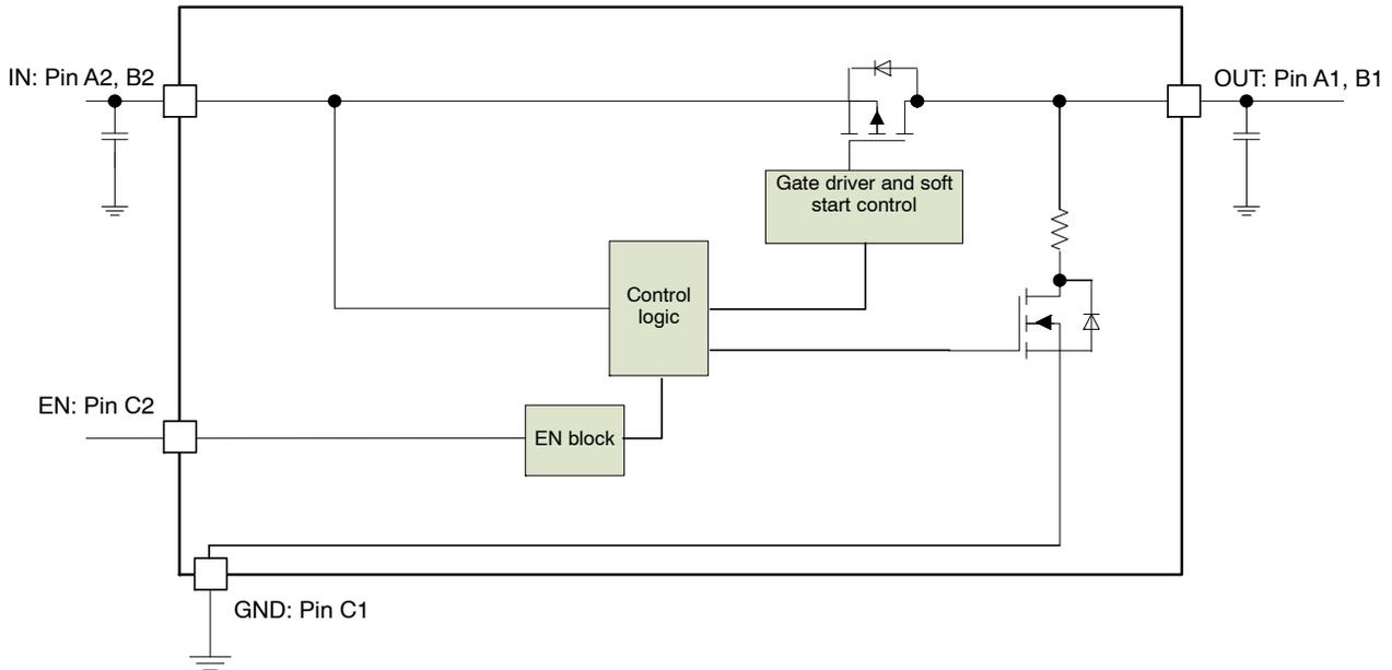
Figure 2. Block Diagram
