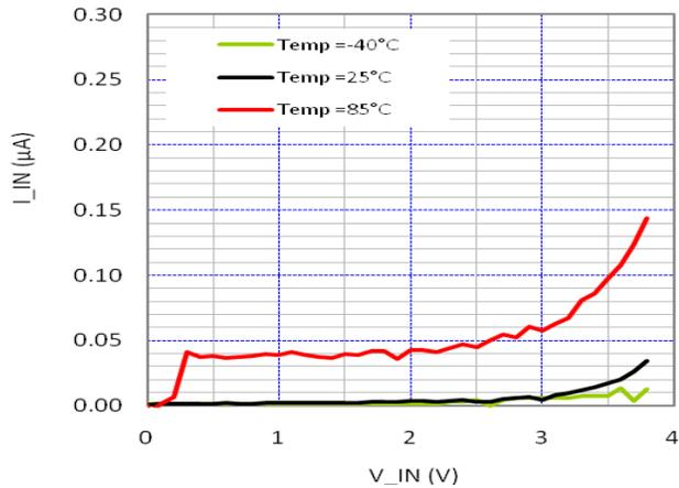
Figure 6. Standby Current ( $\mu A$ ) vs.  $V_{in}$  (V)
