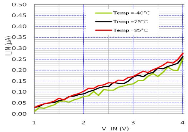
Figure 7. Quiescent Current ( $\mu A$ ) vs.  $V_{in}$  (V)
