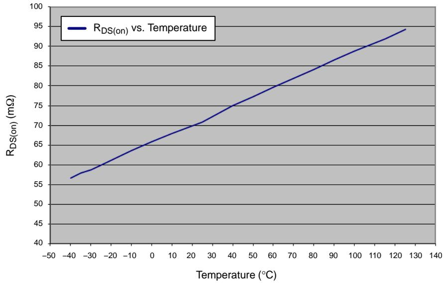
Figure 20. R<sub>DS(on)</sub> vs Temperature, TSOP Package
