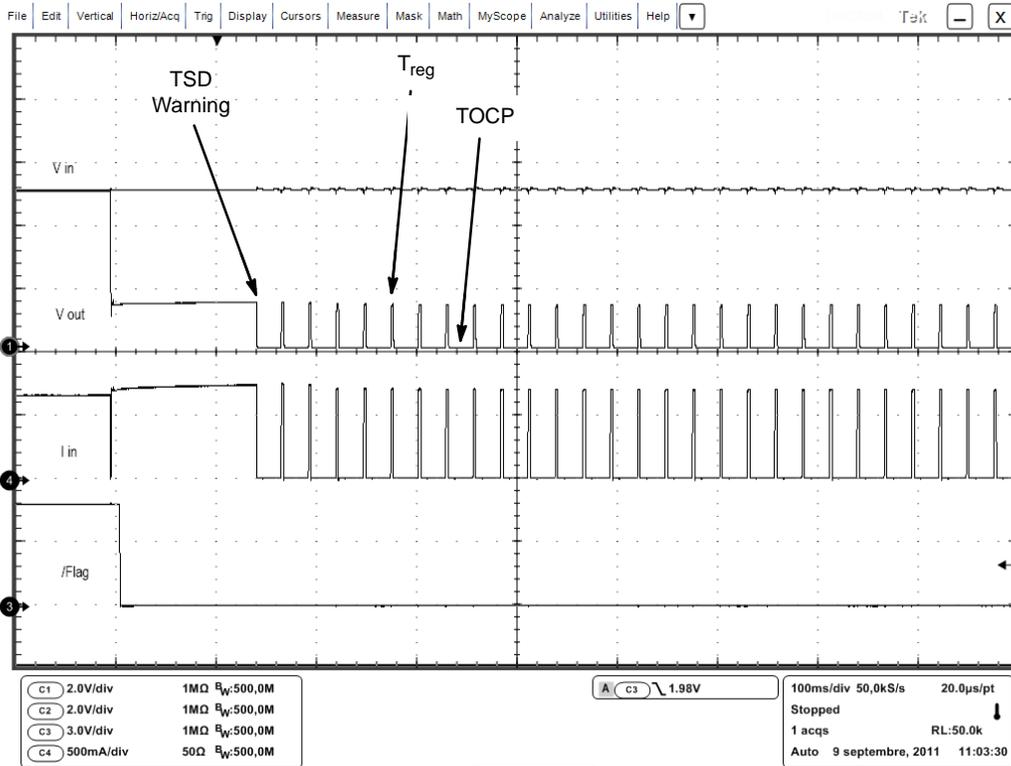
Figure 9. 2 Ω Short on Output. Complete Regulation Sequence
