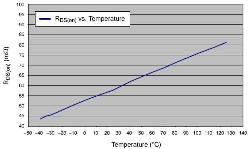
Figure 21. R<sub>DS(on)</sub> vs Temperature, μDFN Package
