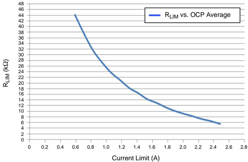
**Figure 25. R<sub>LIM</sub> Curve vs. Current Limit**
