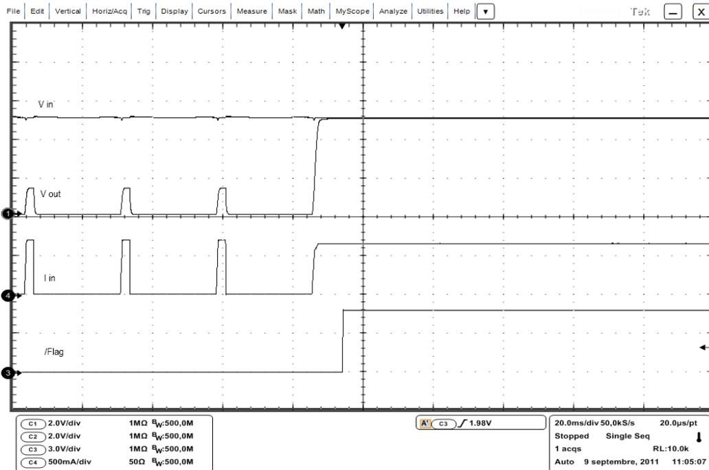
Figure 13. From Timer Regulation to Load Removal Sequence
