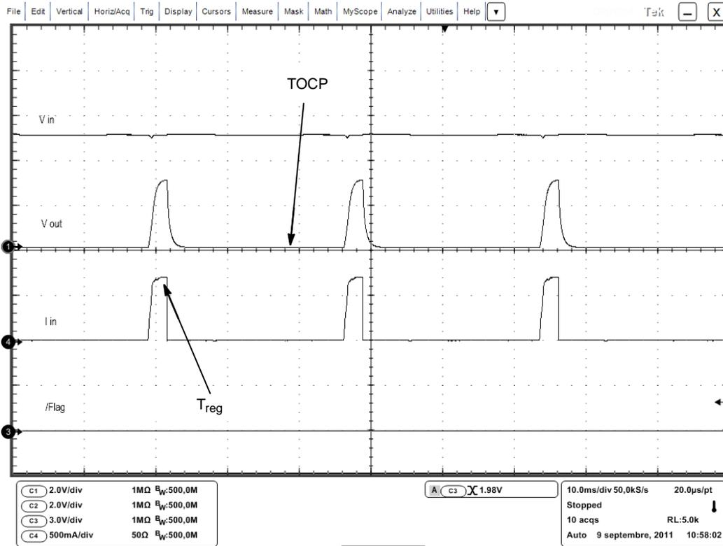
Figure 11. Timer Regulation Sequence During 2 Ω Overload
