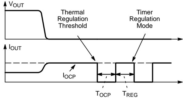
Figure 24. Short circuit
