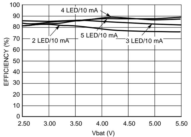
**Figure 11. Overall Efficiency vs. Power Supply –
