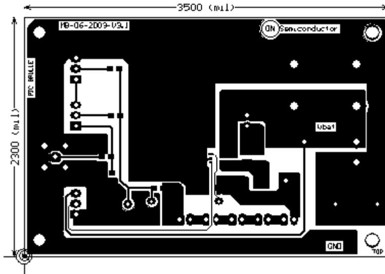
**Figure 33. NCP5007 Demo Board PCB: Top Layer**
