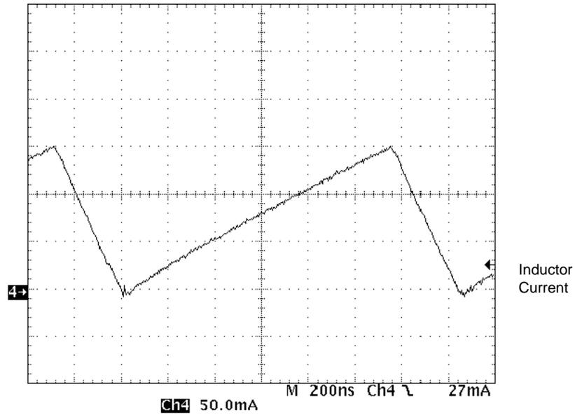
Conditions:  $V_{bat} = 3.6\text{ V}$ ,  $L_{out} = 22\ \mu\text{H}$ , 5 LED,  $I_{out} = 15\text{ mA}$
