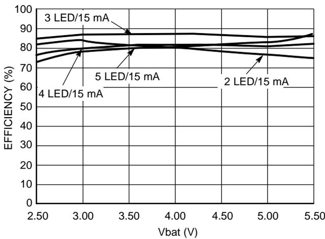
**Figure 12. Overall Efficiency vs. Power Supply –
