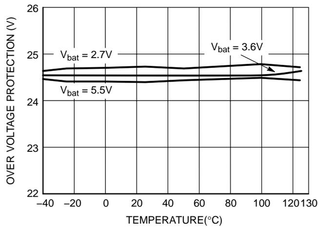
Figure 22. Overvoltage Protection
