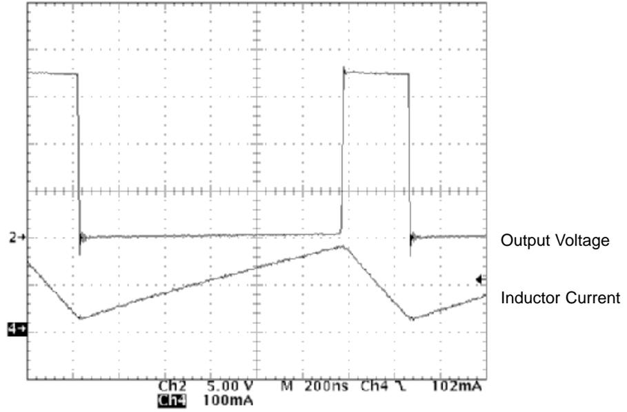
Test Conditions:  $L = 22 \mu\text{H}$ ,  $I_{\text{out}} = 15 \text{ mA}$ ,  $V_{\text{bat}} = 3.6 \text{ V}$ , Ambient Temperature, LED = 5
