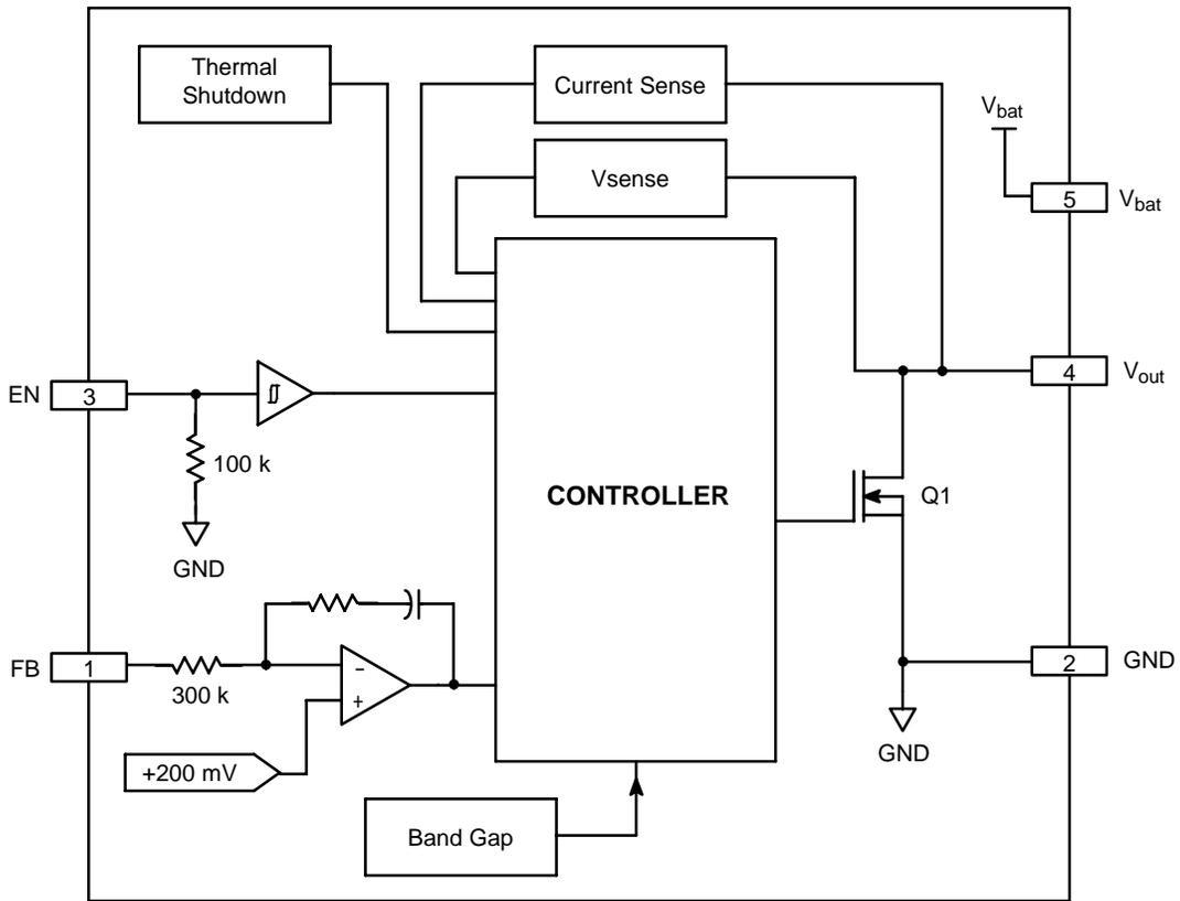
Figure 2. Block Diagram
