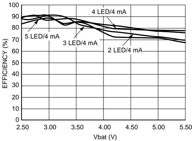
**Figure 10. Overall Efficiency vs. Power Supply –
