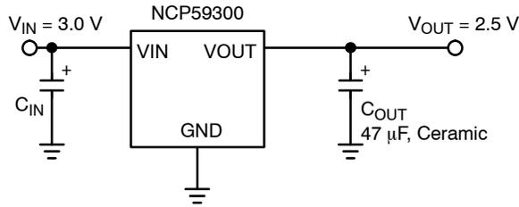
Figure 2. Fixed 2.5 V Regulator in D<sup>2</sup>PAK-3 Package
