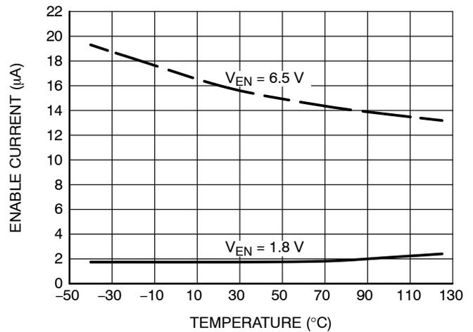
**Figure 14. Enable Pin Input Current vs. Temperature**
