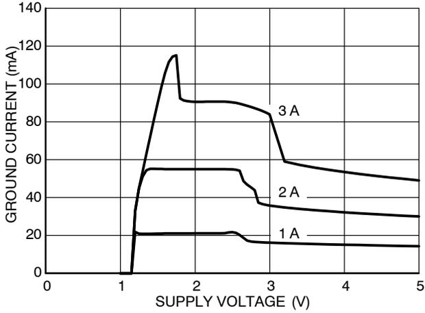
**Figure 9. Ground Current vs. Supply Voltage (2.5 V)**
