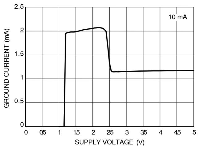
Figure 8. Ground Current vs. Supply Voltage (2.5 V)
