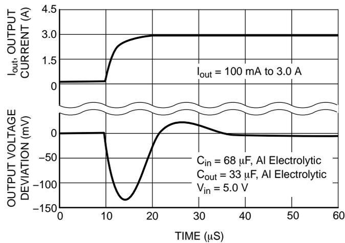
**Figure 12. Load Transient**
